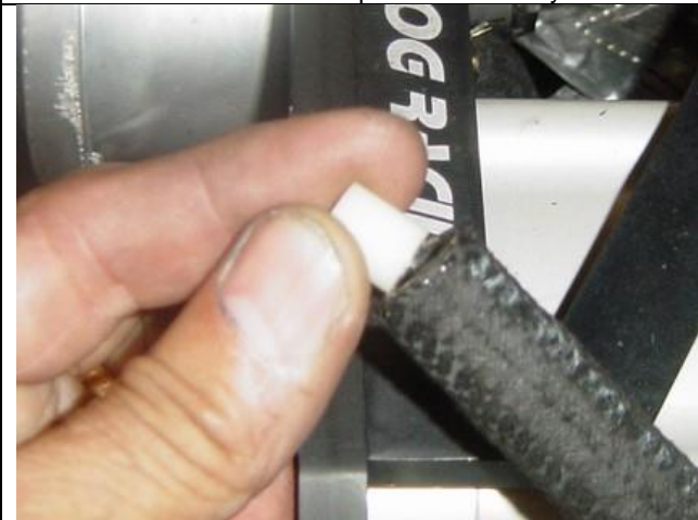
Photo 1-7: Restrictor fitting being installed
