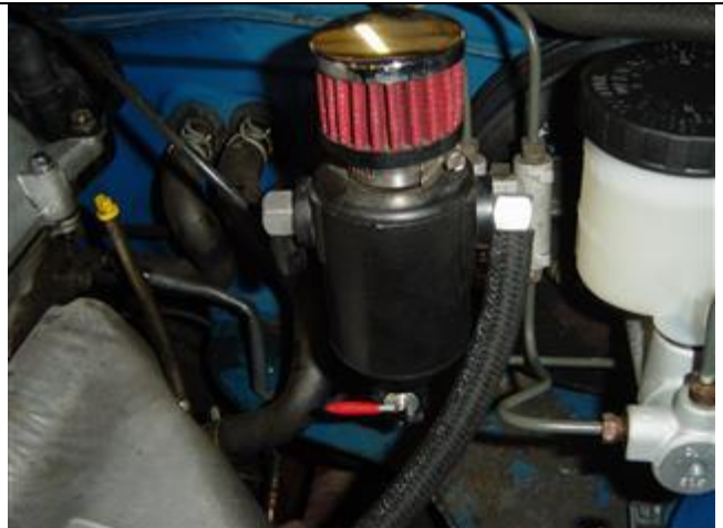
Photo 1-6: Catch can mounted properly
