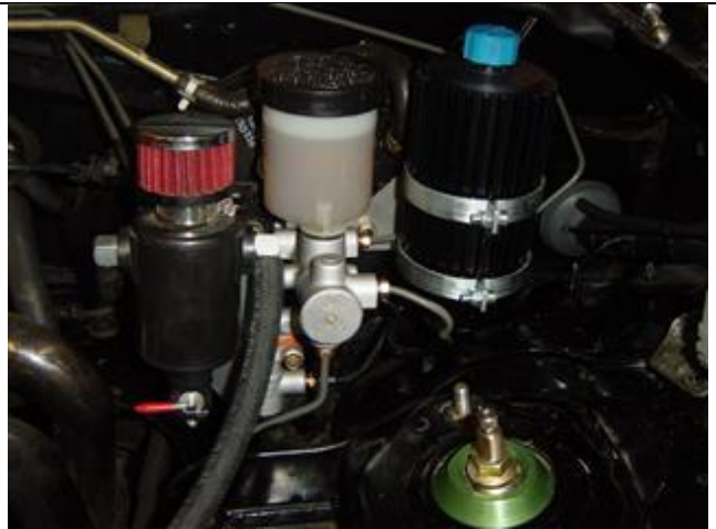
Photo 2-4: Catch installed properly
