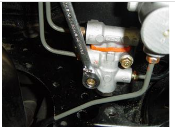
Photo 2-2: Lower bolt removed for catch can install
