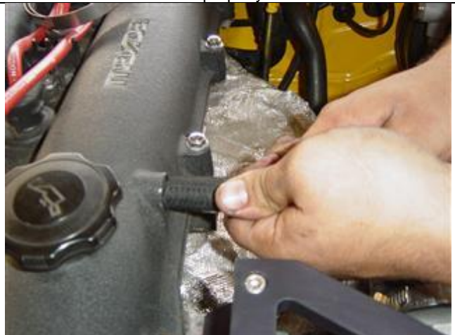
Photo 2-6: Hose installed to valve cover fitting
