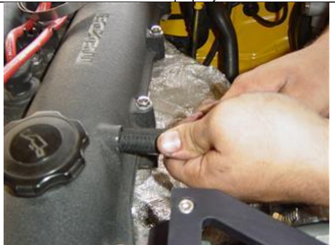
Photo 1-8: Press breather hose onto the valve cover fitting
