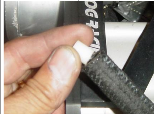
Photo 2-5: Restrictor inserted into hose end
