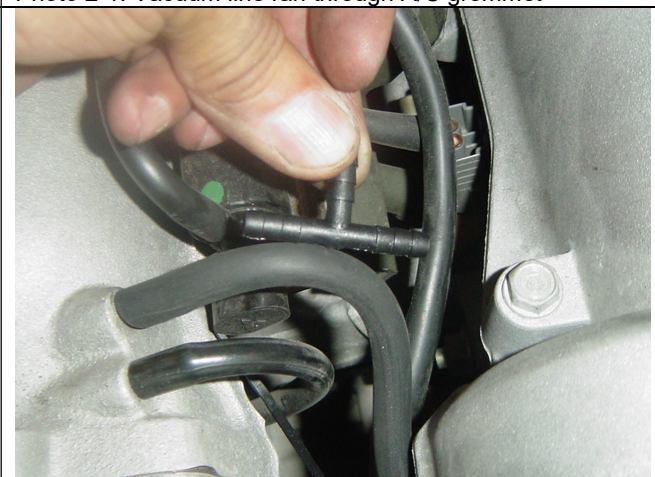
Photo 2-3: Tee fitting for vacuum line
