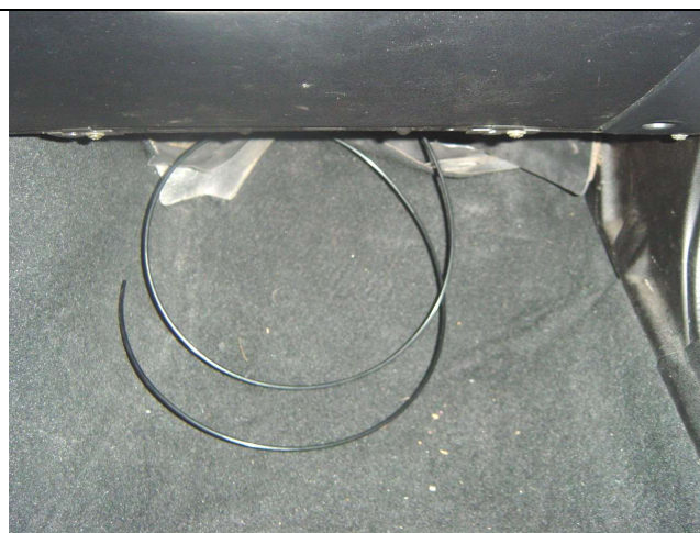
Photo 2-2: Vacuum line pulled through firewall
