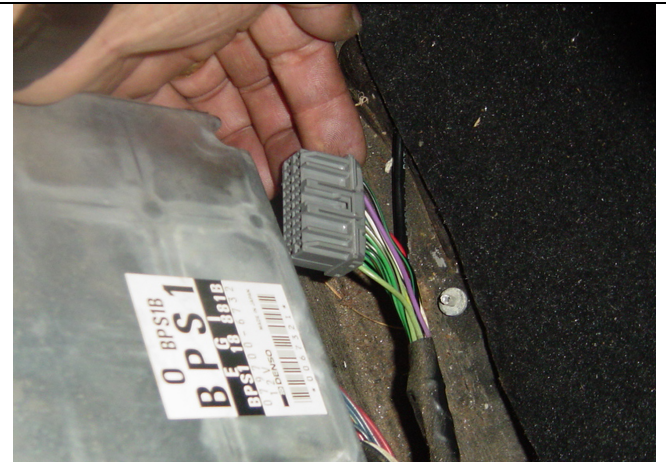
Photo 4-2: Harness removed from ECU
