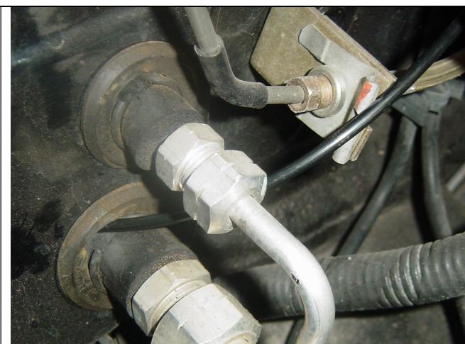
Photo 2-1: Vacuum line ran through A/C grommet
