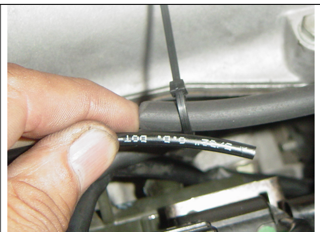
Photo 2-5: Hard line inserted into rubber vacuum line
