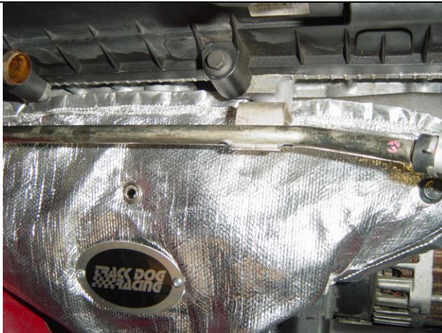
Photo 9: Heat Shield on top side of metal header flange
