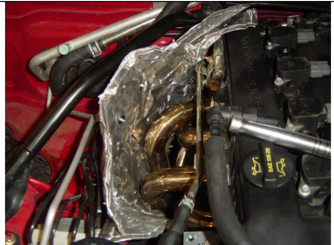
Photo 1-6: Heat Shield between the header and the firewall.
