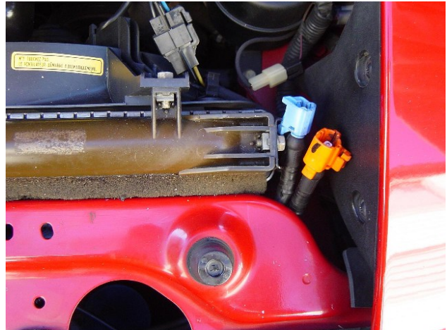
Photo 1-F: Relocate airbag harness under the frame support
