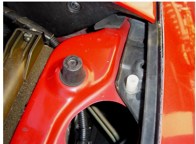
Photo 1-M: Put spacer over the hole
