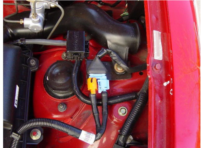
Photo 1-B: Airbag connector on drivers side fender
