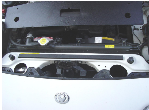
Photo 1-H: Attach the foam gasket
