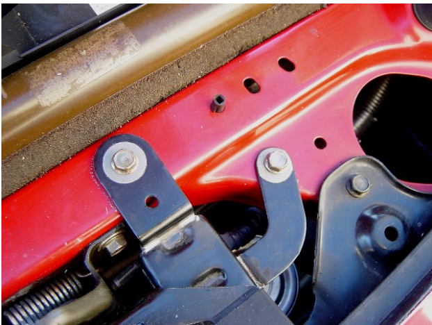
Photo 1-G: Attach the Airbag sensor back to the frame support
