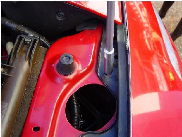
Photo 1-L: Remove 10 mm bolt on each side
