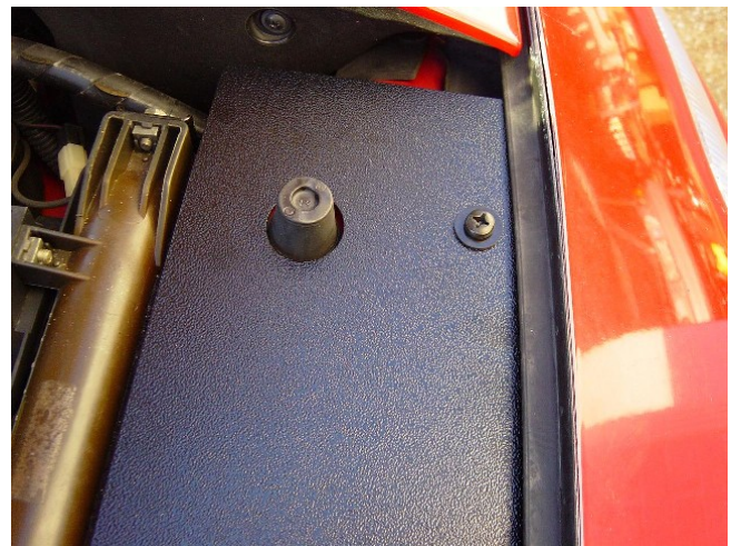
Photo 1-O: Attach screw with washer into hole
