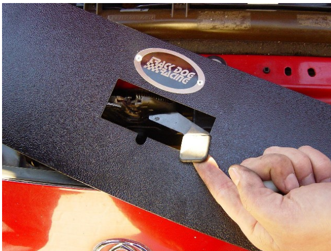
Photo 1-N: Hold latch up during installation
