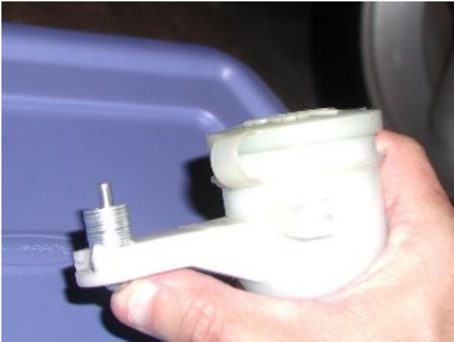
Photo 1-J: Put washers or a spacer the lower the filler
