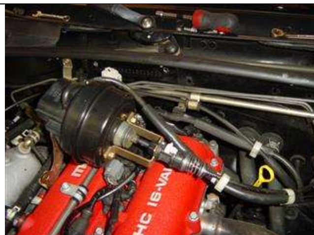
Photo 12-4: Cruise control removed
