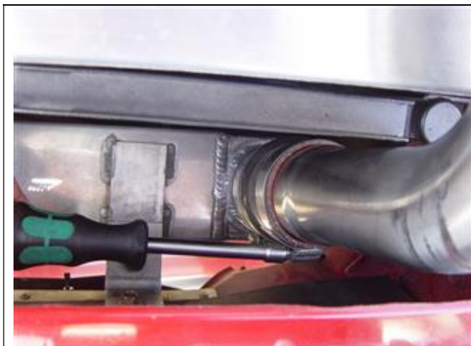
Photo 20-35: Lower clamp tightened
