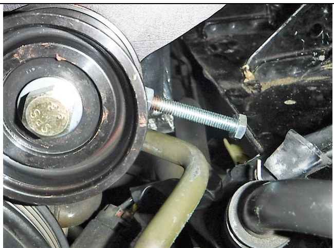
Photo 9-24: Good clearance between hard tube
