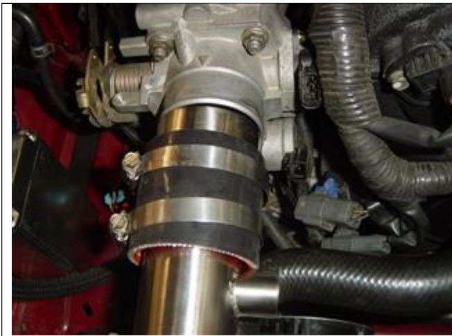
Photo 20-3: Silicone hose and clamps on pipe
