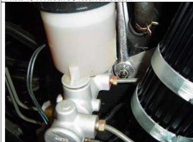
Photo 13-9: Reservoir tightened down to the reservoir
