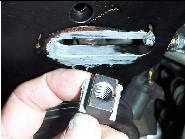
Photo 9-19: Anti-seize on T-nut and slide area
