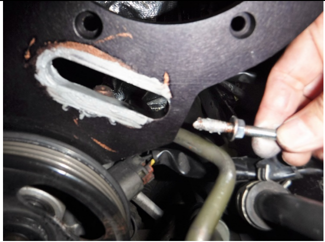
Photo 9-20: Anti-seize on adjustment bolt.
