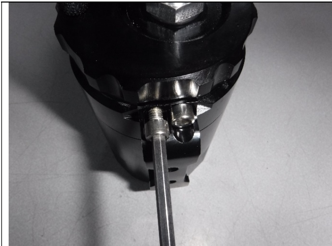
Photo 18-5: Mounting clamp removed
