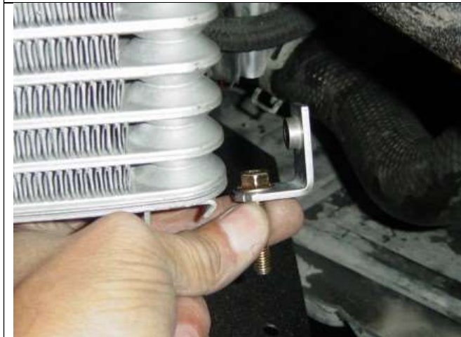
Photo 11-21: Small L-bracket for side panel
