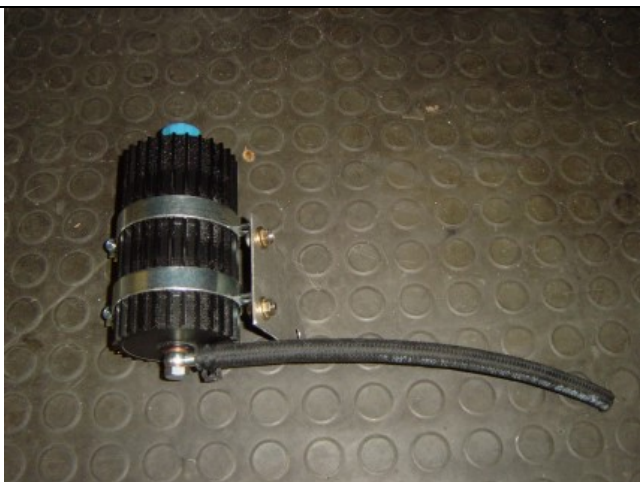
Photo 13-2 Small 12 in. bottom hose on reservoir
