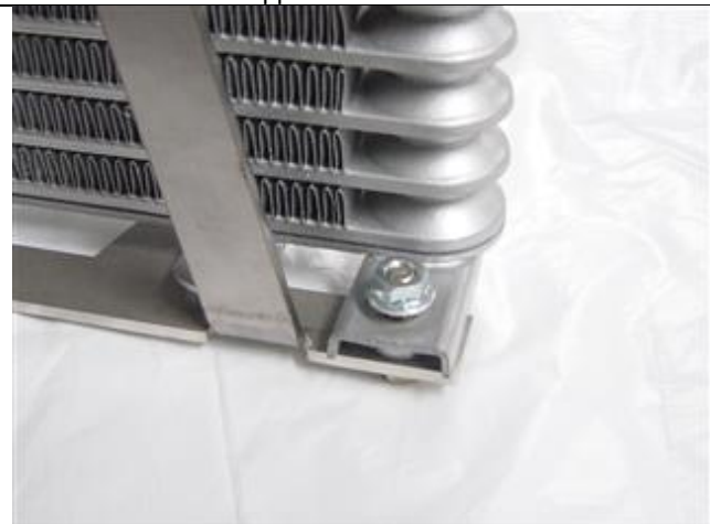
Photo 11-16: Left bottom bolt mounted
