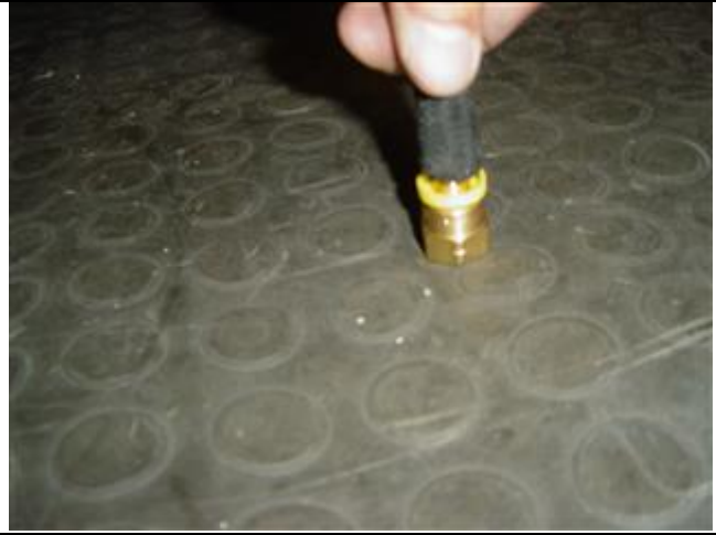
Photo 11-8: Push connector on with extreme pressure
