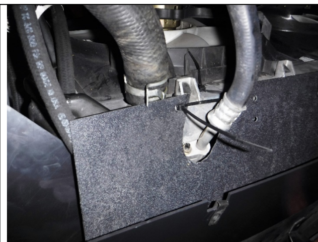
Photo 17-12: Lower 1 panel modified and tie-wrapped
