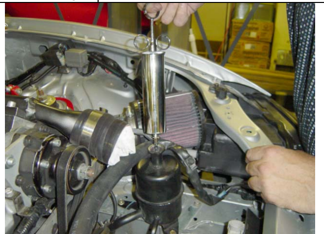
Photo 1-24: P/S fluid sucked from the reservoir.
