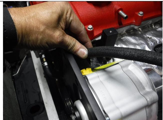
Photo 13-14: Oil hose in position
