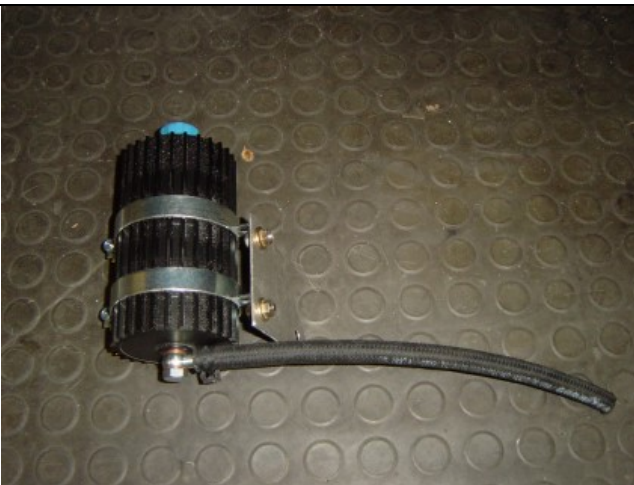
Photo 11-3: 12 inch hose piece to be used for the reservoir
