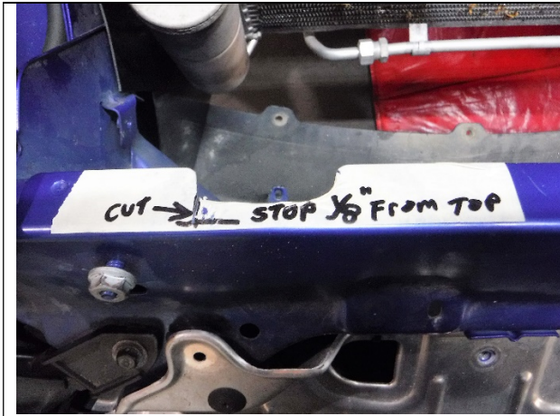
Photo 3-3: Taped for cutting
