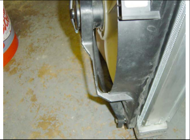
Photo 17-2: Radiator support trimmed for clearance
