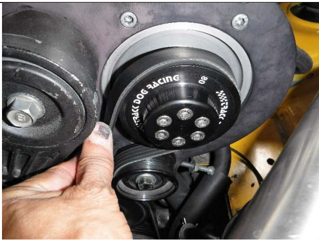
Photo 16-1: Turn tightener bolt out to install belt
