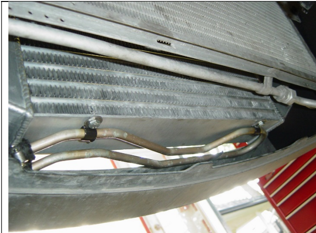
Photo 8-3: P/S tube installed on bottom of intercooler
