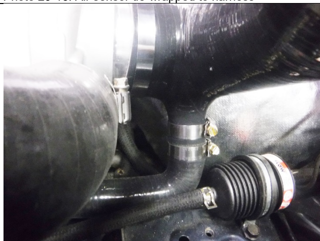
Photo 20-18: BOV return hose attached to intake hose
