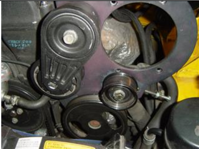
Photo 9-21: Tensioner pulley installed
