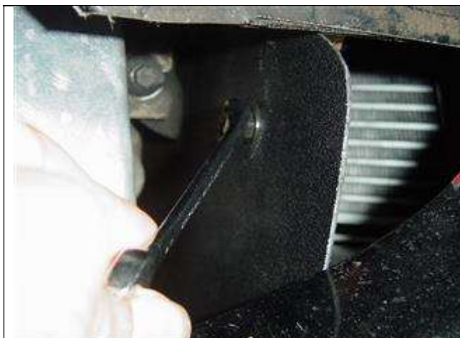
Photo 6-9: Front M6 bolt tighten on side panel
