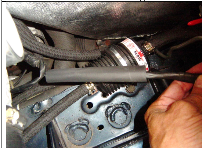
Photo 19-13: Shrink tubing slid over crimp connectors
