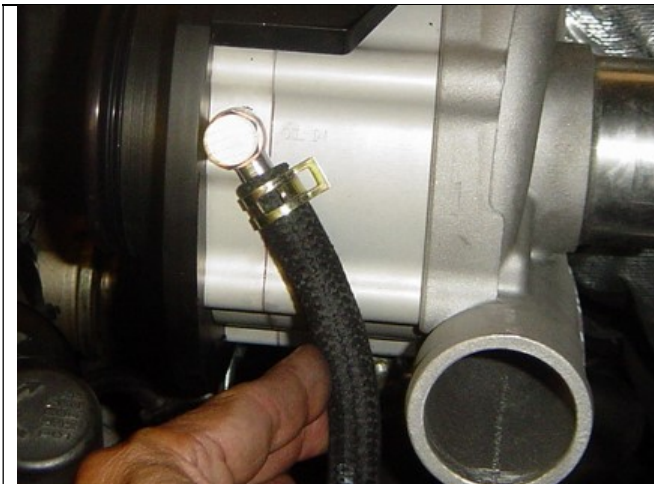
Photo 22-3: Hose connector loose for bleeding oil
