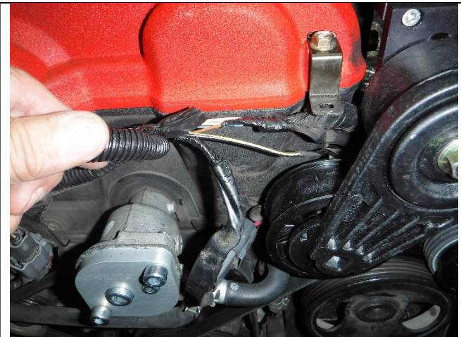
Photo 10-10: Crank sensor wiring pulled out of harness
