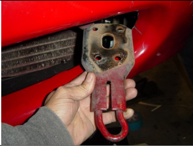
Photo 11-1: Left side tow hook removed
