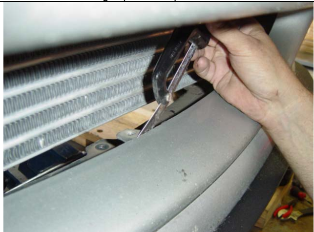
Photo 1-20: Plastic tabs removed from bumper
