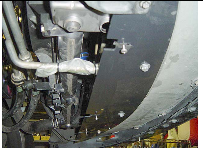
Photo 8-6: Lower 2 panel installed
