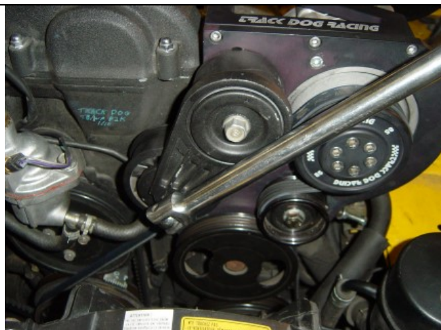
Photo 16-4: 3/8" breaker bar used to remove tension
