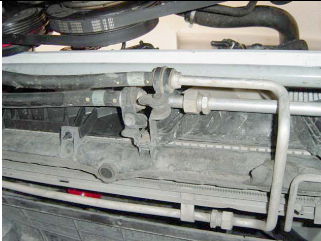
Photo 1-11: A/C bracket removed
