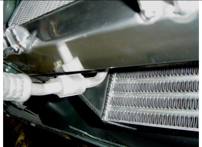
Photo 5-12: Check clearance and bend the A/C line under the radiator
