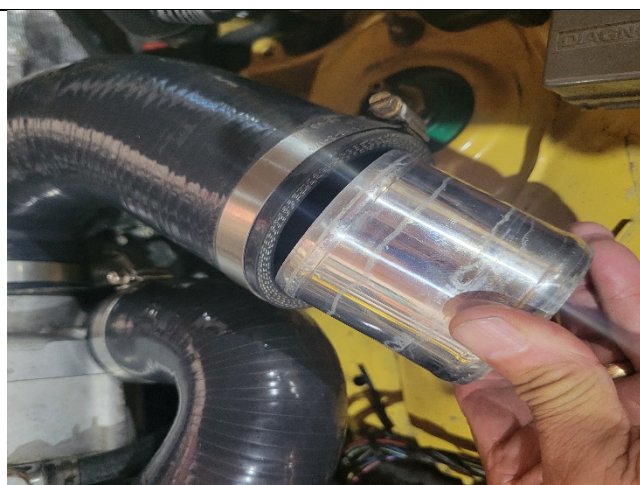
Photo 20-20: Metal pipe insert
