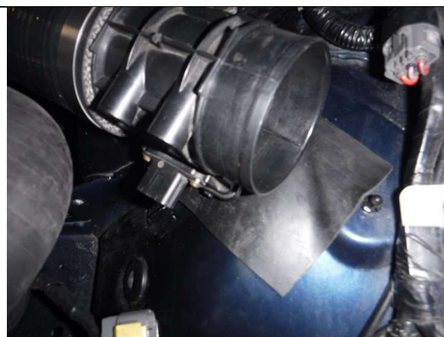
Photo 20-30: MAF over rubber pad
