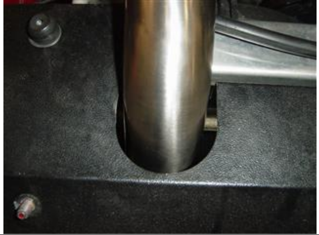
Photo 20-6: Radiator cover clearance checked
