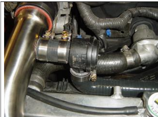
Photo 20-9: BOV return air system
