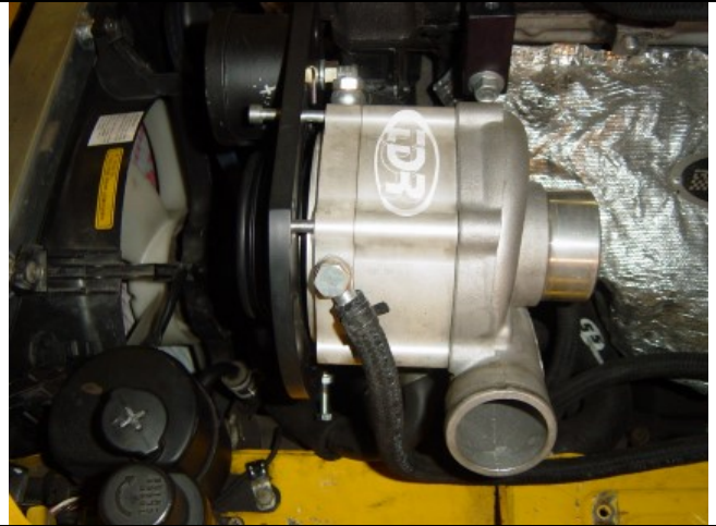
Photo 13-20: Filter hose attached the SC
