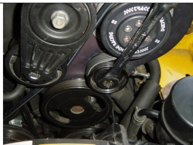
Photo 16-6: Tighten slider pulley with 14 mm wrench
