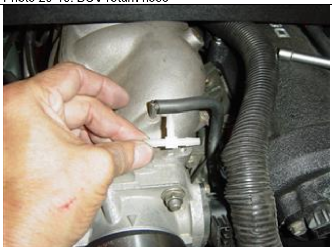
Photo 20-12: Vacuum line from BOV to intake manifold
