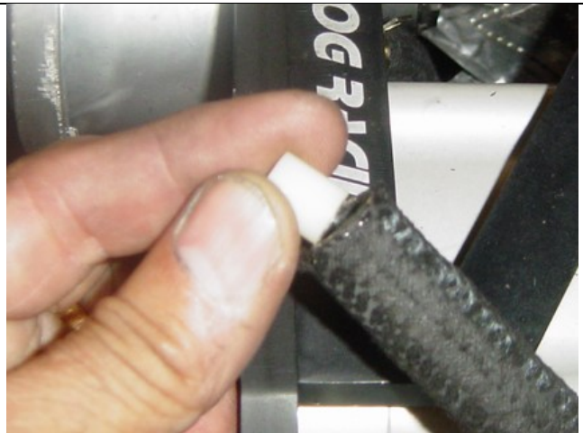
Photo 18-20: Restrictor fitting being installed
