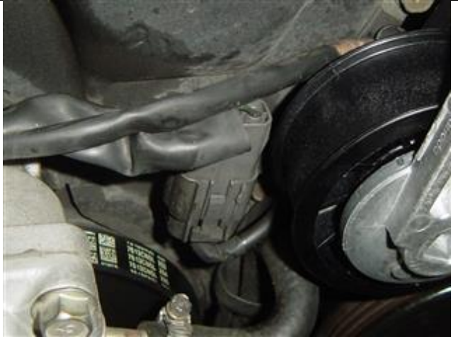
Photo 10-2: Crank sensor connector to be repositioned
