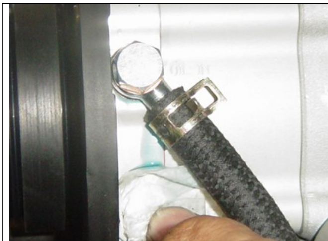
Photo 22-7: Oil pushed into Rotrex inlet
