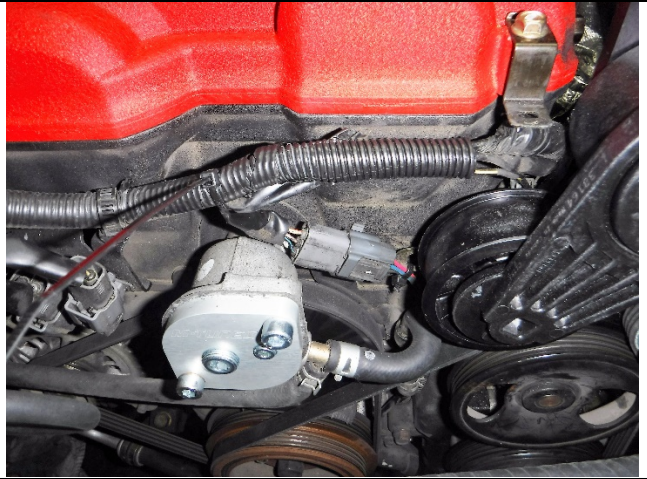
Photo 10-12: Crank harness tie-wrapped
