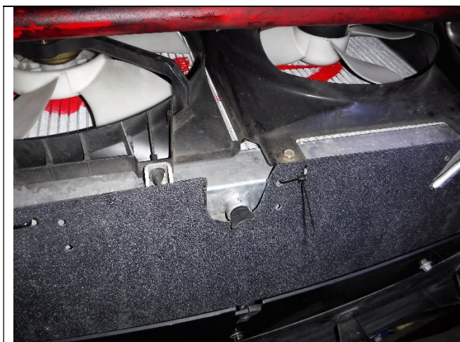
Photo 17-11: Lower 1 panel modified and tie-wrapped
