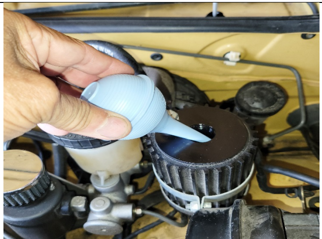
Photo 22-4: Reservoir pressure fitting with bulb
