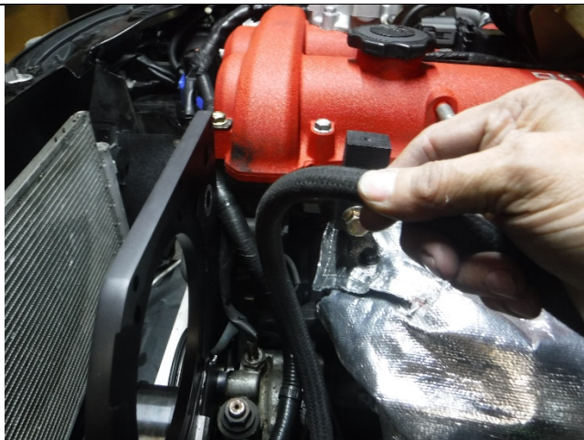
Photo 13-13: Oil hose from oil cooler
