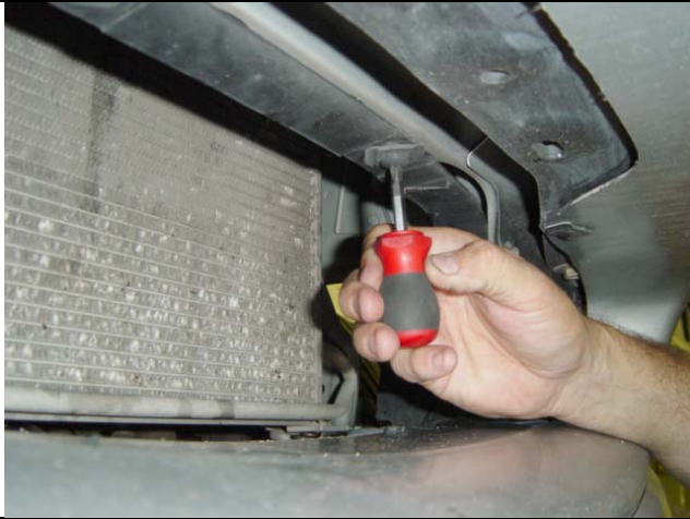
Photo 1-15: Cowling screws removed
