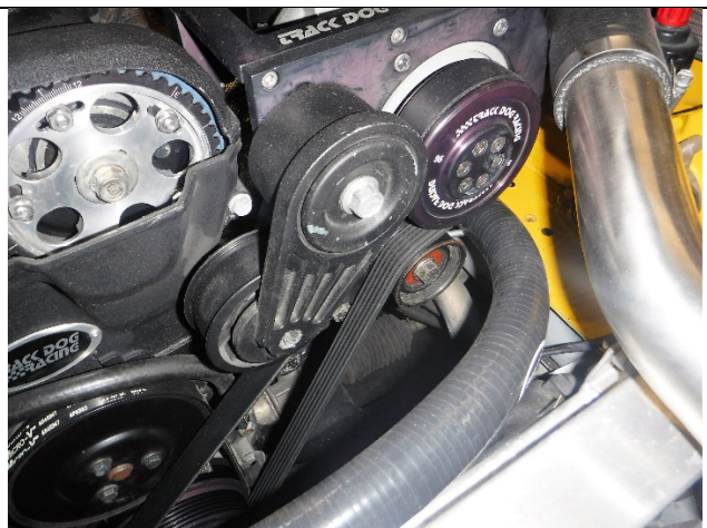
Photo 16-10: 6-rib setup installed
