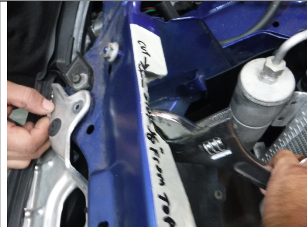
Photo 3-9: Crescent wrench used to bend left end
