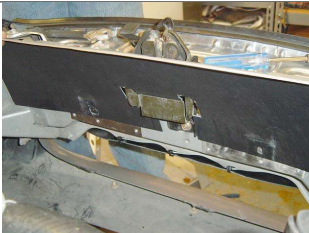
Photo 6-13: Upper 1 panel bent at tabs and Upper 2 panel
