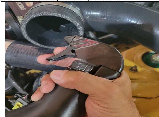
Photo 20-17: Add soapy water to aid installation
