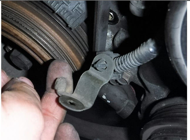
Photo 10-4: Lower crank sensor bracket removed
