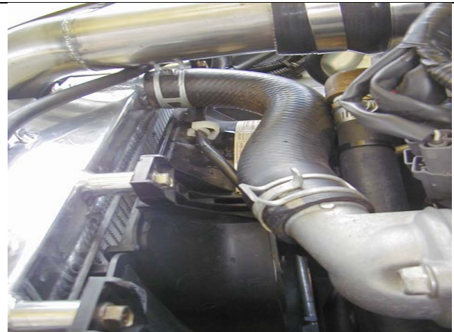
Photo 17-4: Upper radiator hose trimmed to fit
