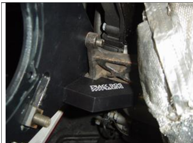
Photo 9-15: P/S block installed
