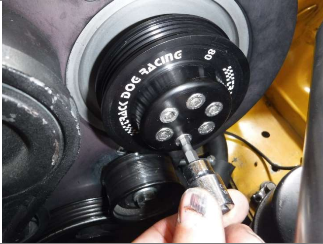
Photo 15-3: Remaining Allen bolts installed
