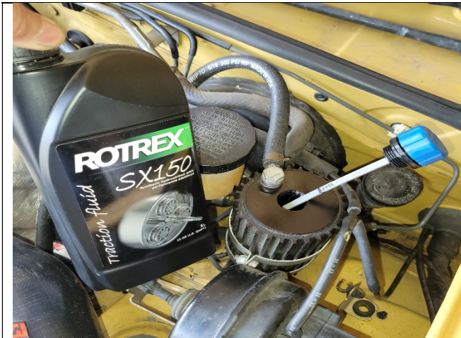
Photo 22-1: Rotrex oil to be poured into reservoir
