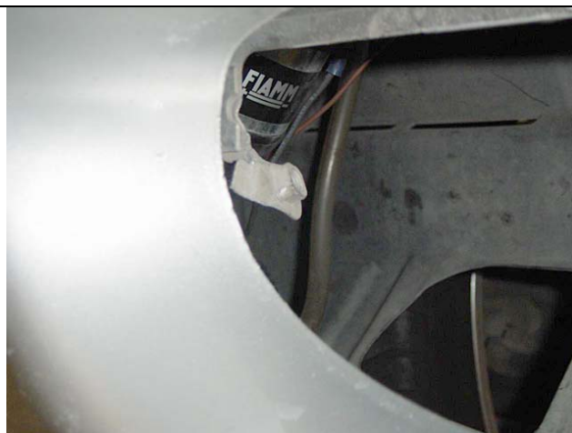
Photo 6-2: Metal bracket bent back 90 degrees
