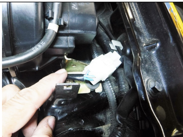
Photo 21-4: Cruise control reconnected
