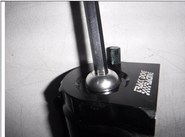
Photo 18-1: Cap removed from top with Allen wrench
