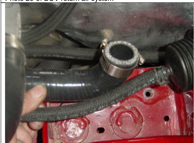
Photo 20-11: BOV return hose with clamp
