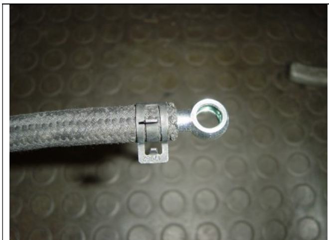
Photo 13-3: Fitting installed with spring clamp
