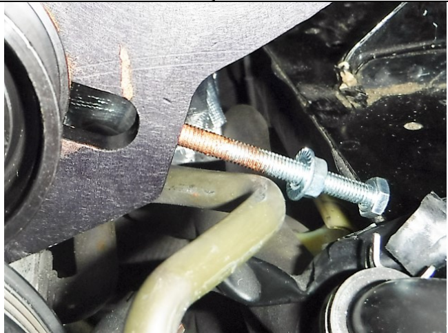
Photo 9-22: Clearance checked P/S hard line
