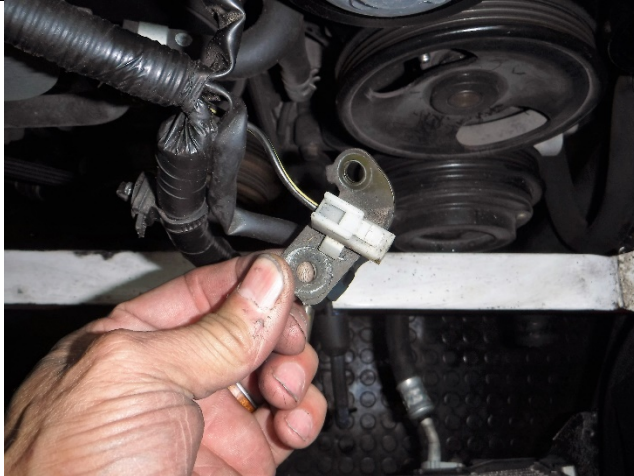
Photo 10-1: A/C switch bracket removed
