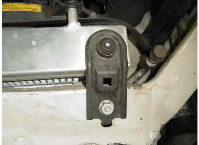
Photo 1-2: Upper radiator bracket
