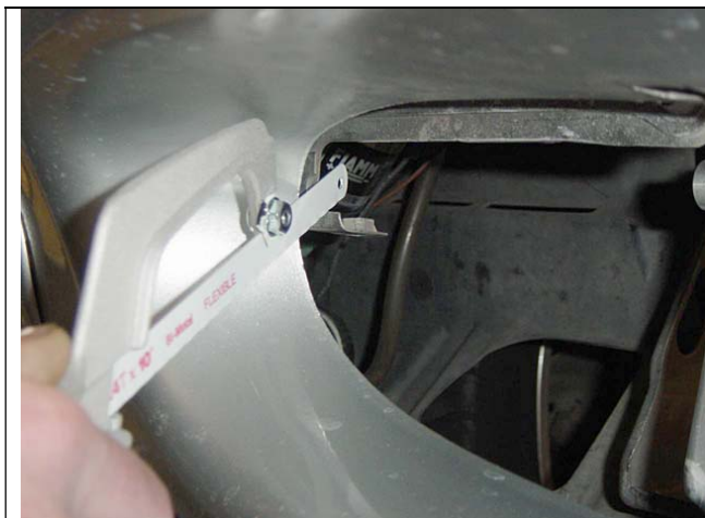
Photo 6-1: Metal bracket cut with hack-saw
