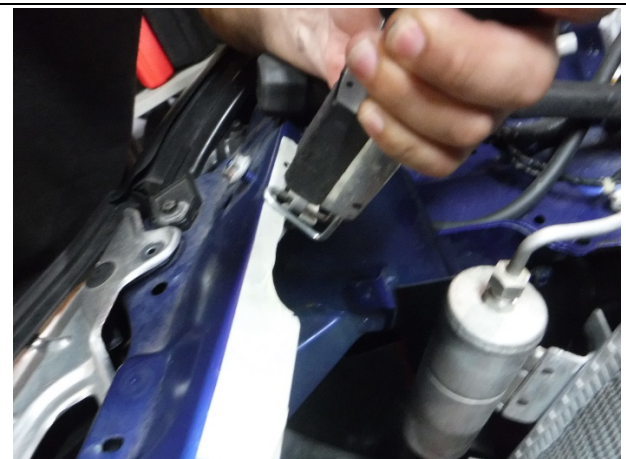
Photo 3-6: Jig-saw cutting the cross member
