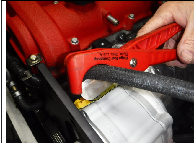
Photo 13-15: SC outlet hose cut
