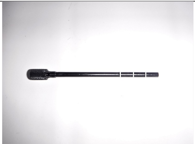
Photo 18-24: Dip stick oil level marks
