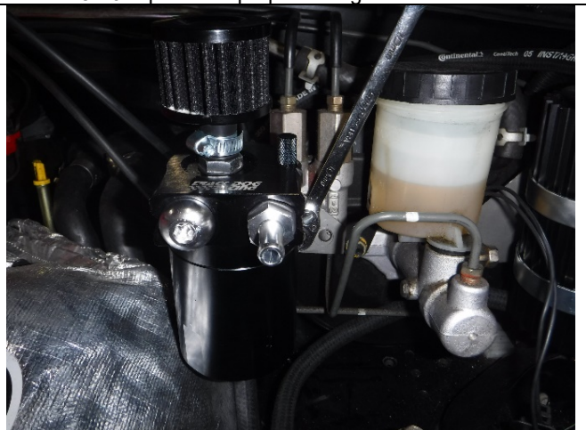
Photo 18-12: Catch can installed
