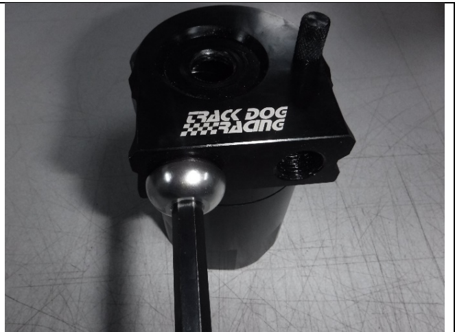
Photo 18-2: Cap installed on left side of catch can
