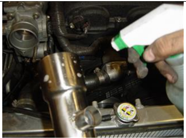
Photo 20-4: Soapy water applied on pipe
