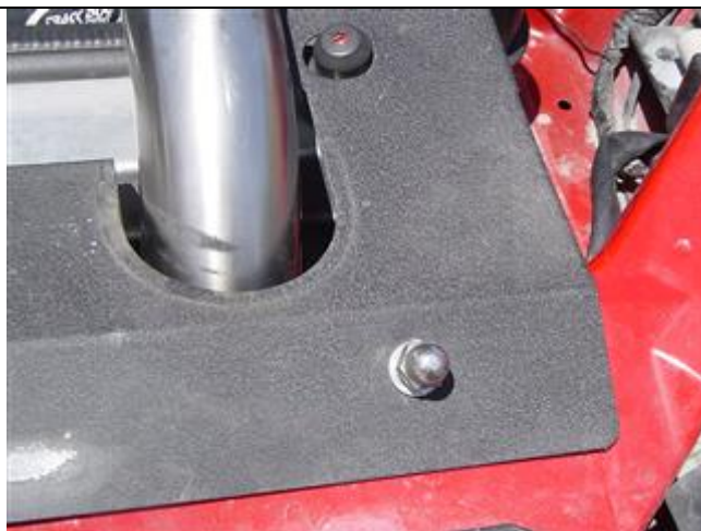
Photo 20-36: Radiator cover installed
