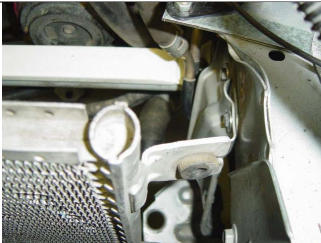
Photo 17-7: Bracket bent towards radiator
