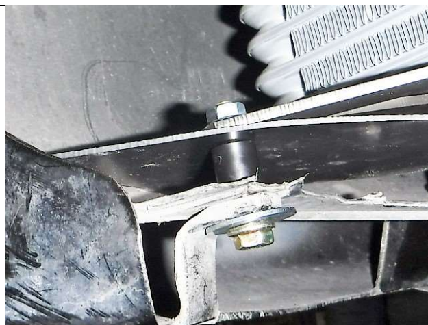
Photo 11-20: Cooler bracket mounted to bumper
