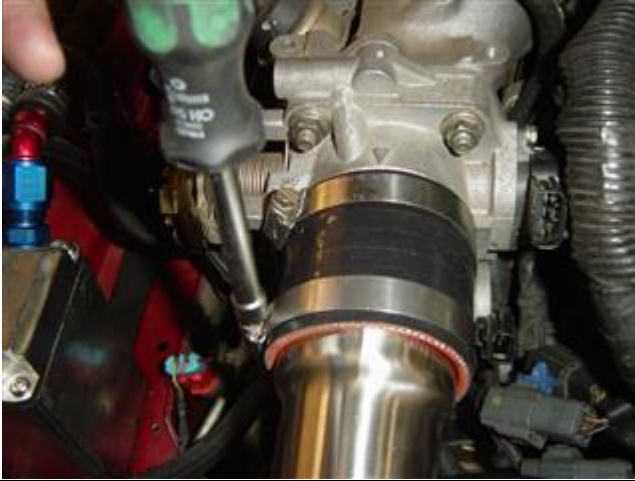
Photo 20-5: Tighten TB clamp first and align
