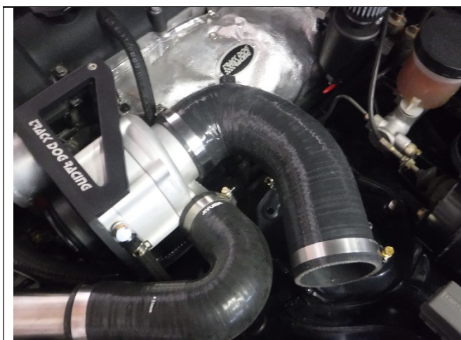
Photo 20-19: Supercharger intake hose
