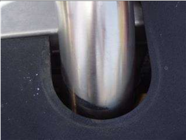
Photo 20-34: Pipe centered through radiator cover
