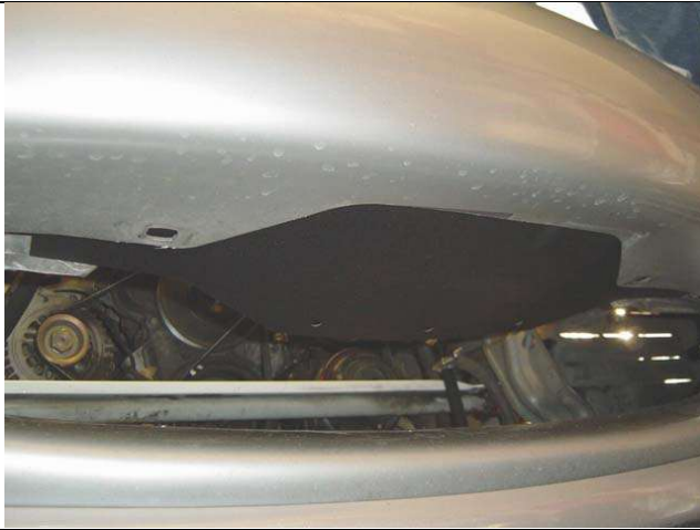
Photo 6-11: Upper 1 panel slipped into bumper
