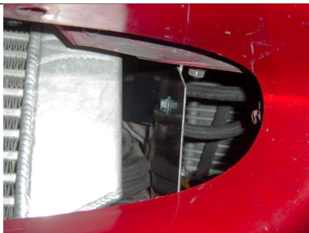
Photo 6-10: Side panel installed as air diffuser
