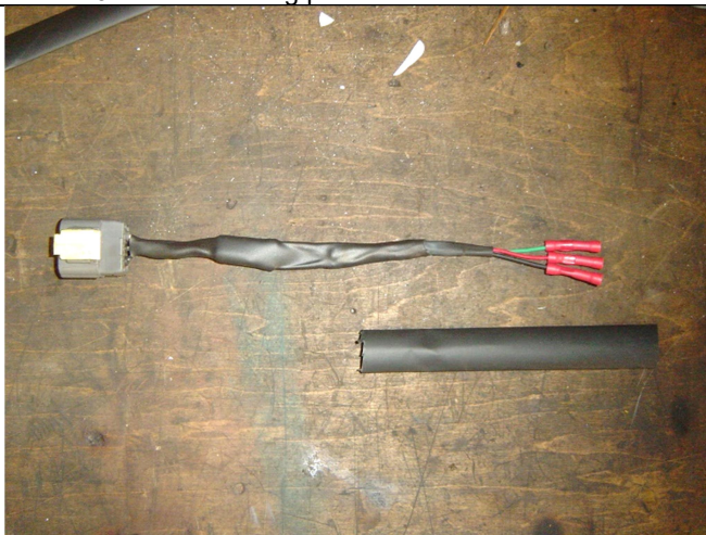
Photo 19-9: Connector end complete
