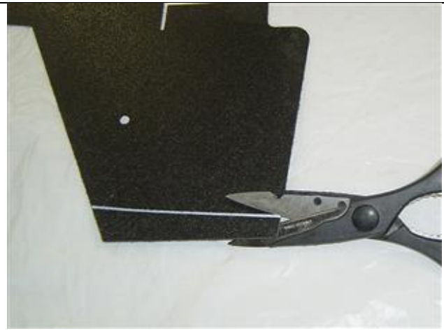
Photo 6-6: Panel cut to be used as air diffuser
