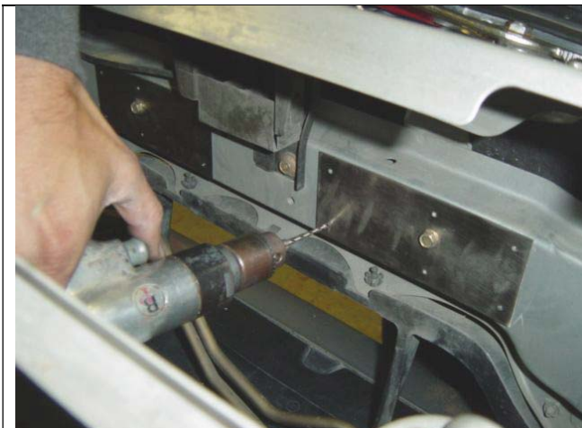
Photo 4-1: Drill 1/8" holes using the plate as a guide
