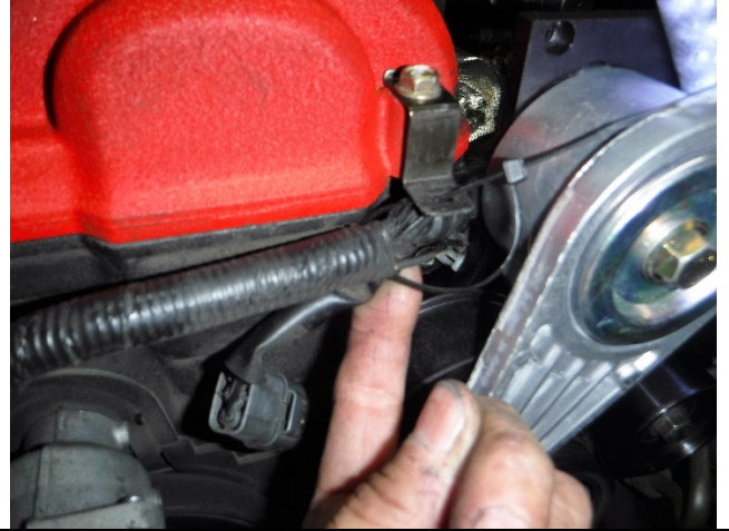
Photo 10-8: Harness pulled up and tie-wrapped
