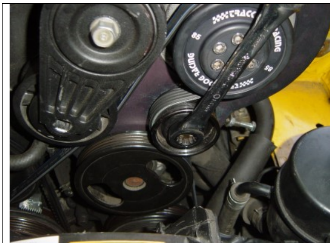
Photo 16-3: Sliding pulley uses 14 mm wrench
