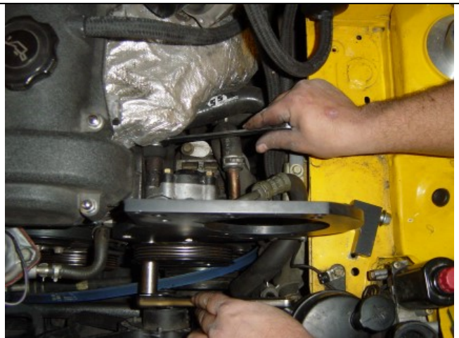
Photo 9-6: Tighten lower bolts on bracket
