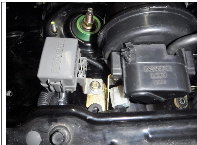
Photo 21-3: New diagnostic mount with cruise control
