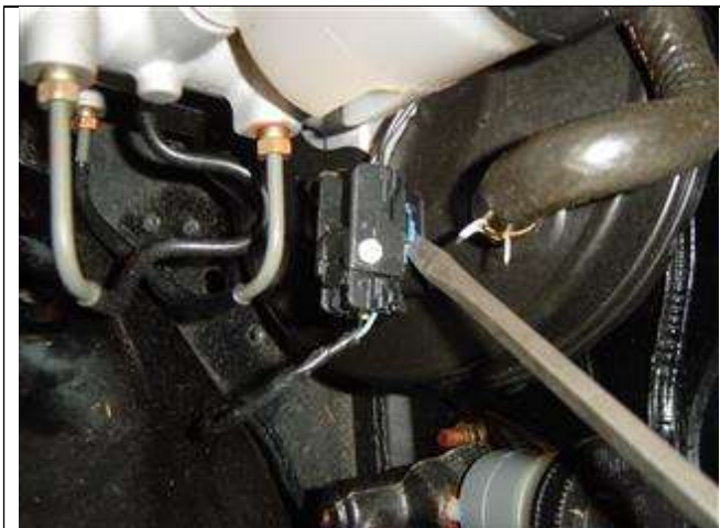
Photo 12-1: Electrical connection on 01-05 model
