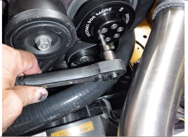
Photo 15-4: After belt installed bolts tightened
