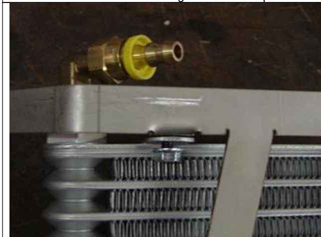
Photo 11-15: Upper hardware mounted to oil cooler
