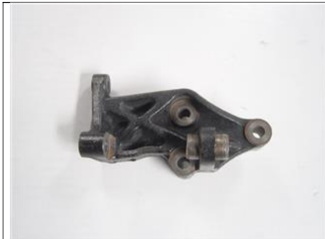
Photo 1: Factory power steering mount all year models
