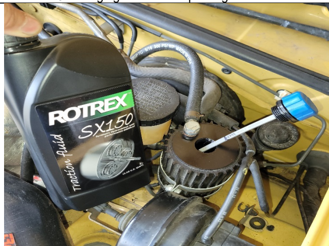
Photo 22-10: Dip stick reading
