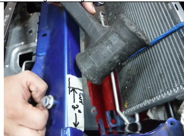
Photo 3-8: Rubber mallet used to bend cross member
