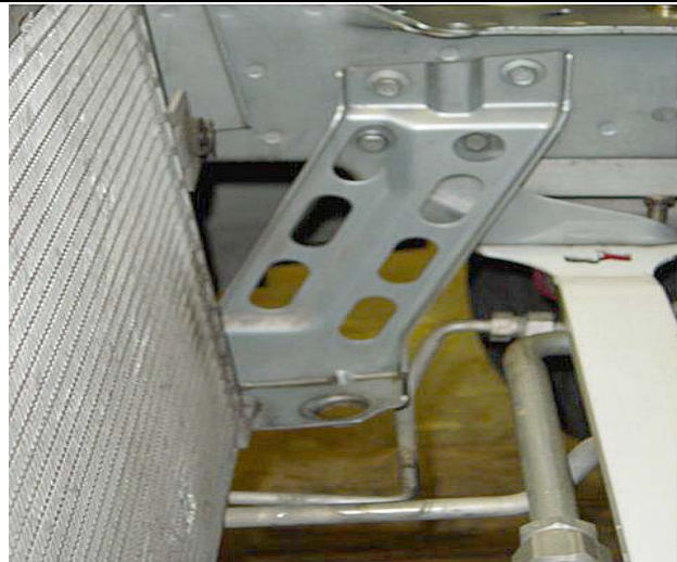
Photo 2-1: Stock mounted radiator mount
