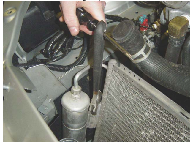
Photo 5-4: Bending canister using crescent wrench on top
