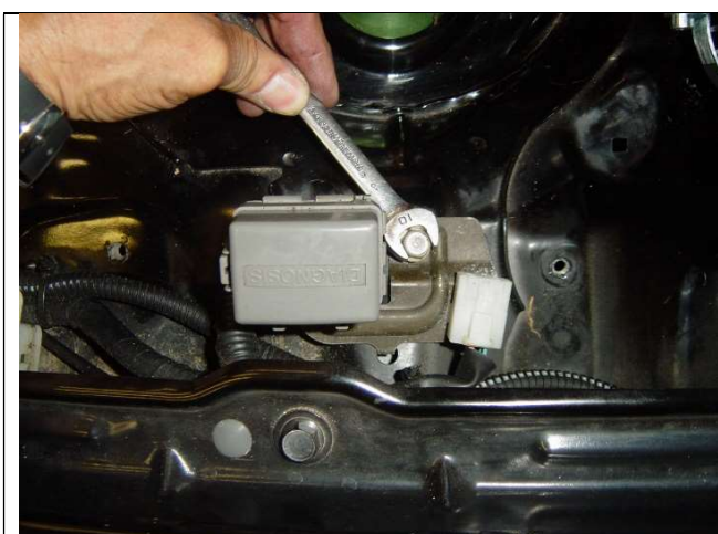
Photo 12-5: Diagnostic mount removed
