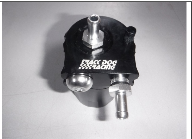
Photo 18-4: 3/8" hose fitting front, 7/16" hose fitting top
