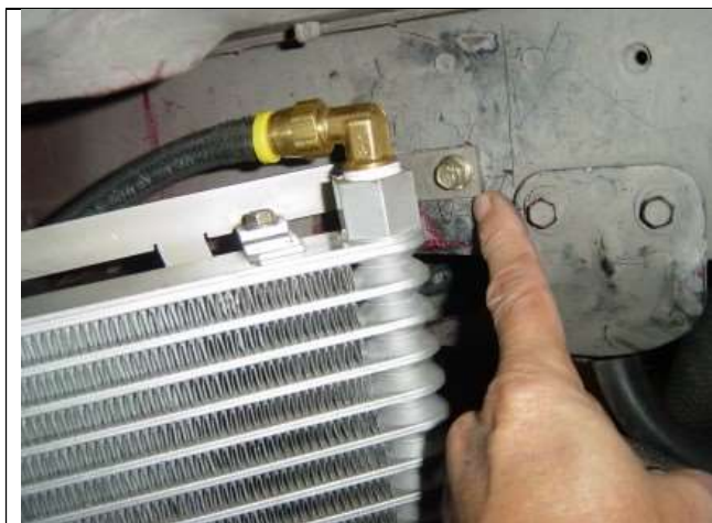
Photo 11-19: Cooler mounted to frame
