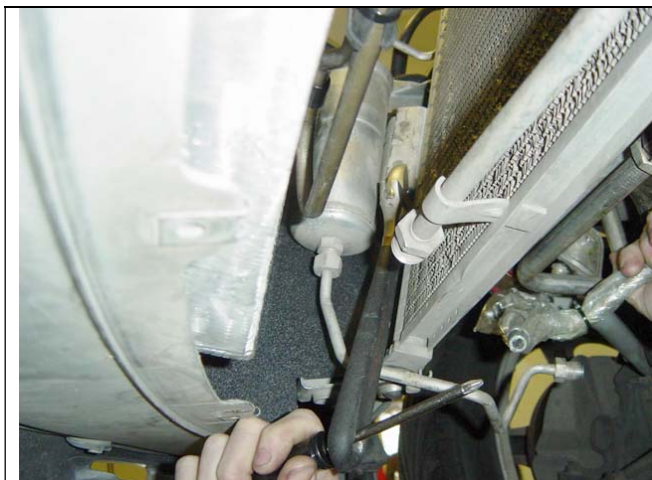
Photo 5-5: Bending canister using crescent wrench on bottom
