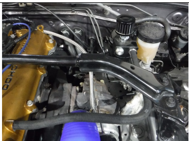
Photo 18-18: Catch can complete
