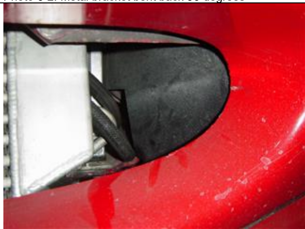
Photo 6-4: Side panel installed with no airflow to oil cooler
