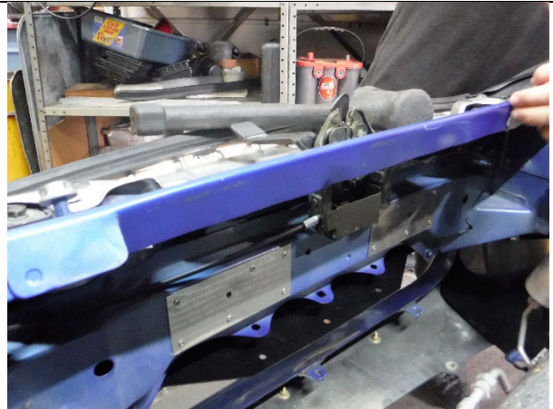
Photo 3-10: Cross member bent vertical
