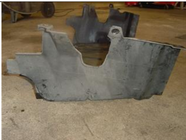
Photo 11-9 Belly pan before modification
