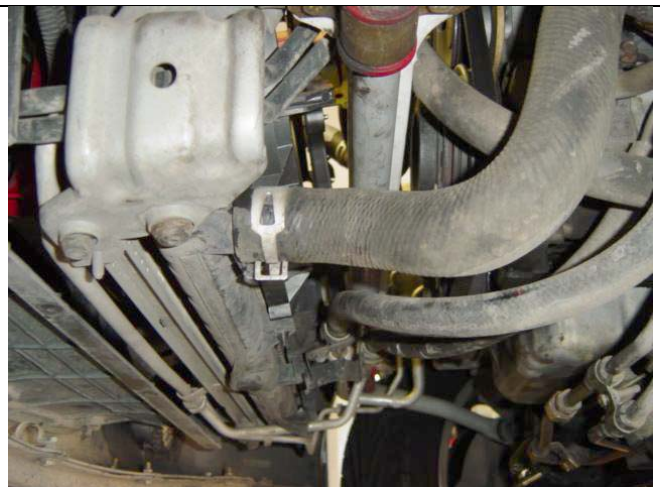
Photo 1-10: Lower radiator hose and support
