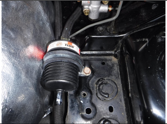
Photo 13-12: Oil direction with filter mounted
