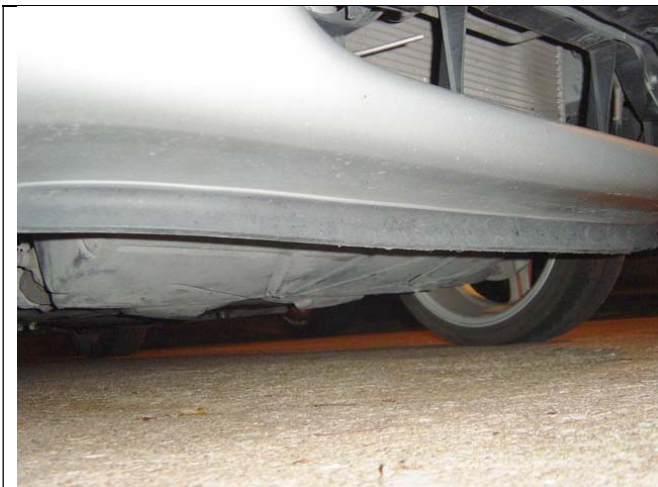
Photo 1-9: Front lip spoiler under the bumper
