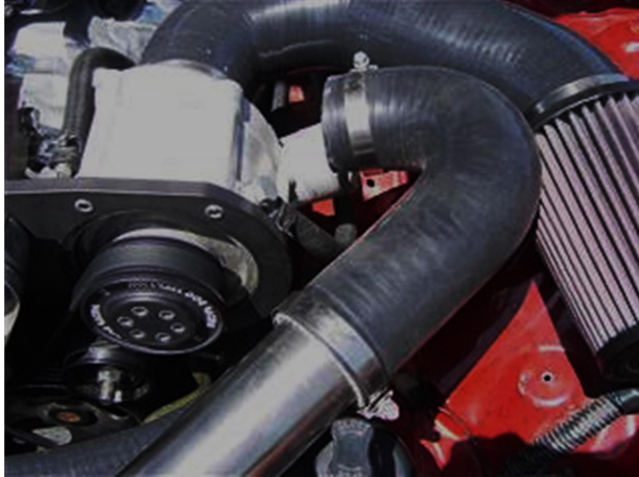
Photo 20-31: Supercharger outlet hose
