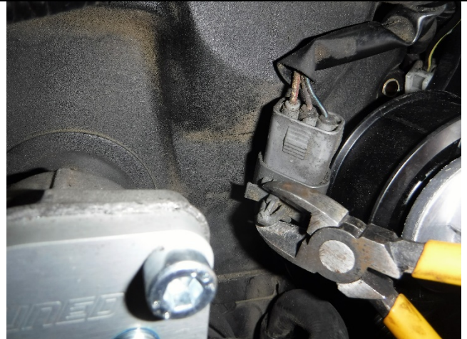
Photo 10-6: Push-in mount cut off for clearance
