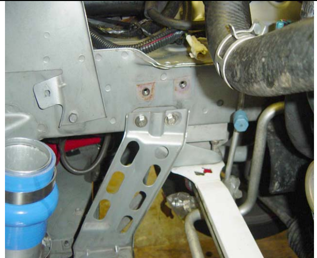
Photo 2-2: Radiator mount in new position
