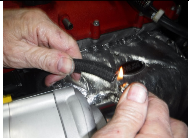
Photo 13-16: Burning off the threads
