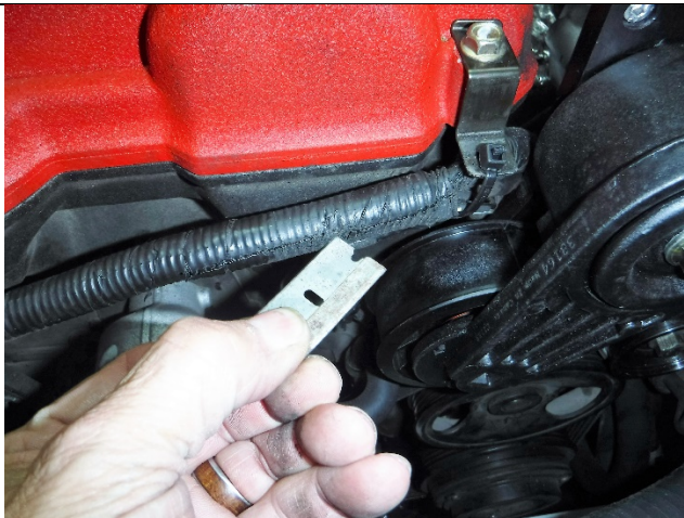
Photo 10-9: Wire loom opened to separate wiring
