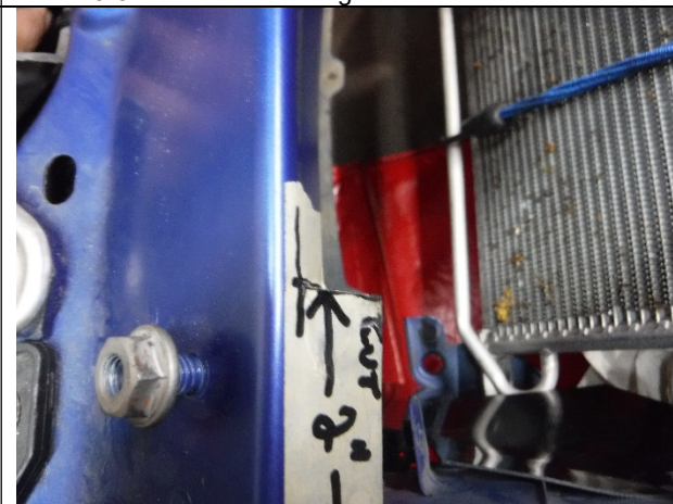
Photo 3-7: Left section cut
