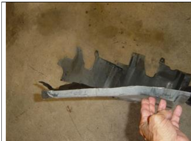
Photo 11-11: Side panel removed about 1 inch from bottom
