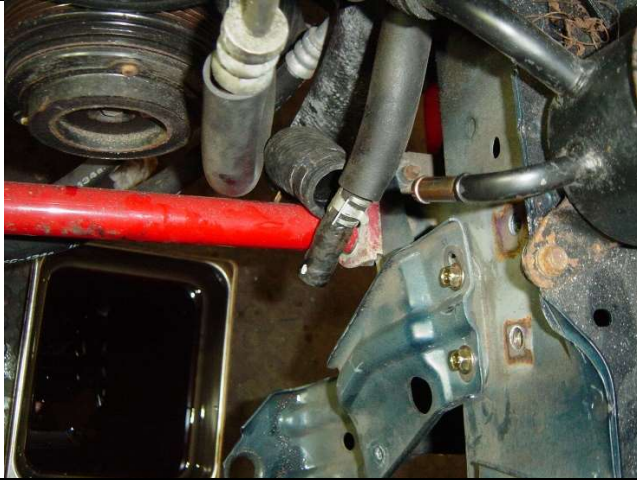
Photo 1-25: Cooling tube fluid removed with drip pan
