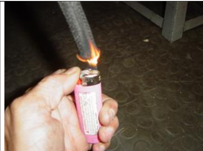
Photo 18-19: Burn fraying on the hose end
