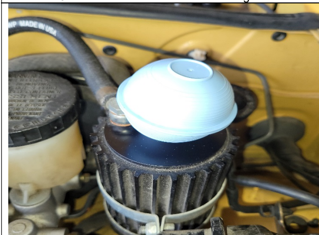
Photo 22-5: Pressure fitting pressed into reservoir opening
