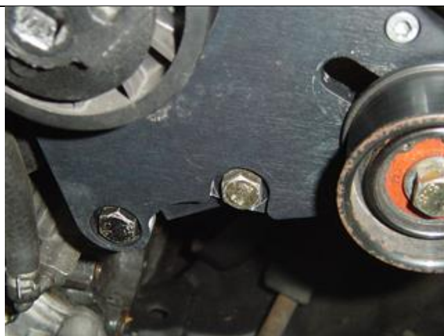
Photo 9-16: Front bolt installed in P/S block
