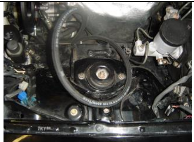
Photo 11-4: Cloth hose pulled through the sway bar mount
