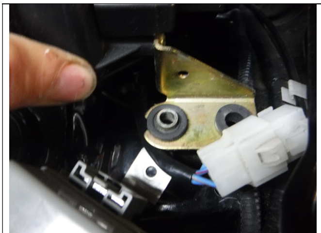
Photo 21-1: Grommet and insert to be removed
