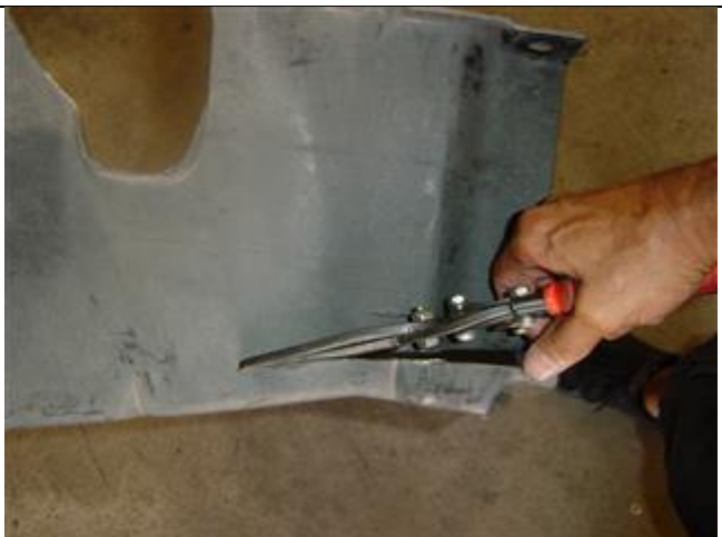
Photo 11-10: Using tin-snips cut side panels off both sides
