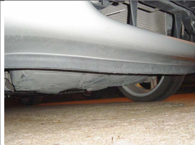
Photo 8-5: Lower factory air dam to be removed
