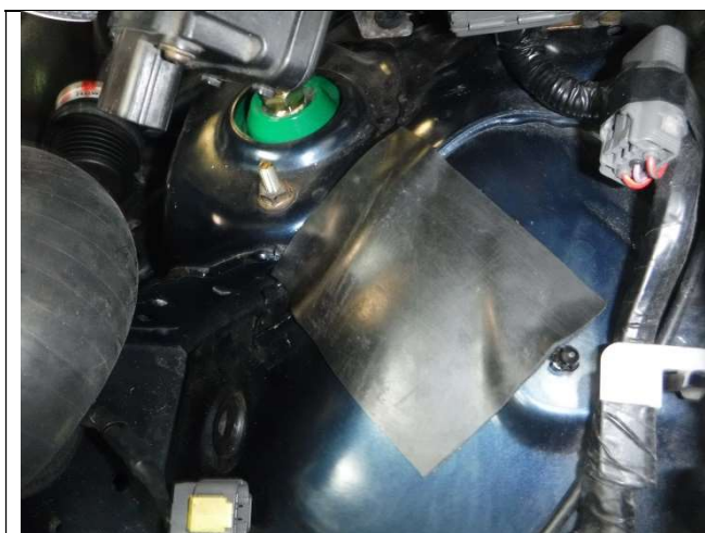
Photo 20-29: Rubber pad installed
