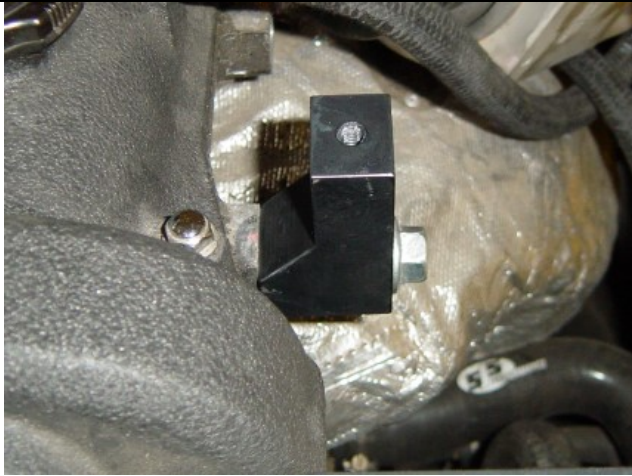
Photo 9-7: Head block assembly
