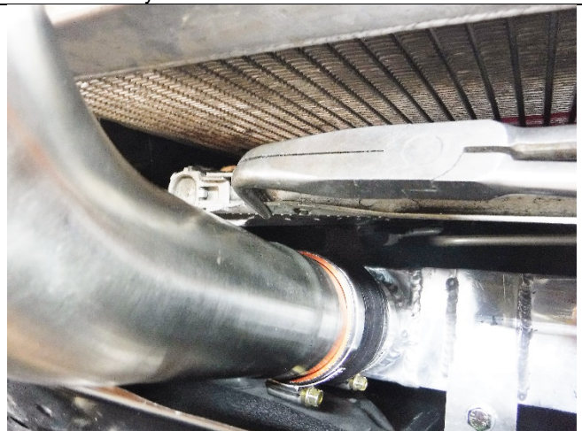
Photo 5-20: Top area bent back using needle nose pliers
