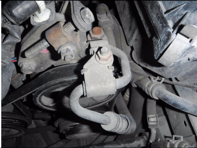
Photo 9-1 P/S hose bracket to be removed
