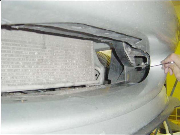
Photo 1-17: Cowling front bolts
