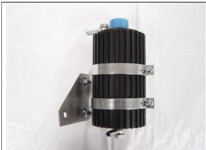
Photo 13-1: Reservoir with mount installed
