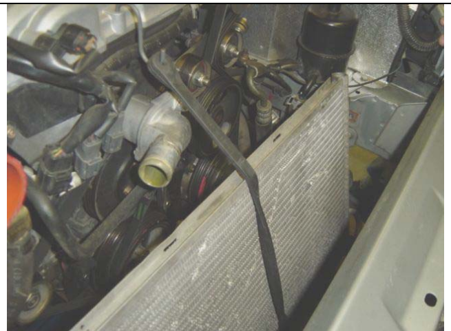
Photo 1-14: A/C condenser strapped back
