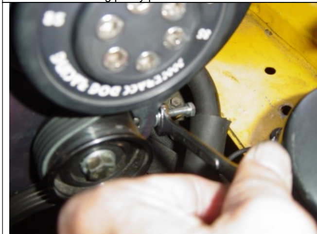
Photo 16-7: Tighten the sliding pulley to tension the drive belt. Lock jam nut when complete
