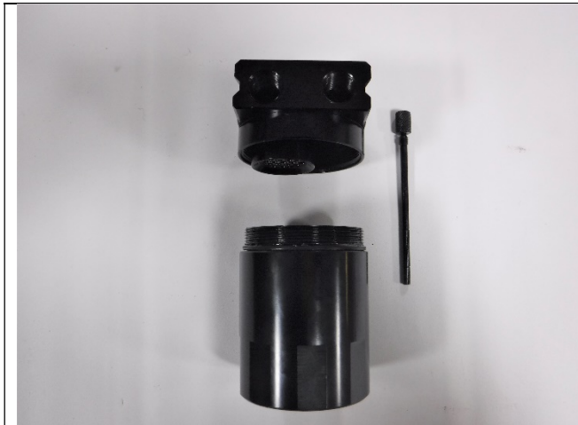
Photo 18-23: Catch can reservoir and dip stick removed
