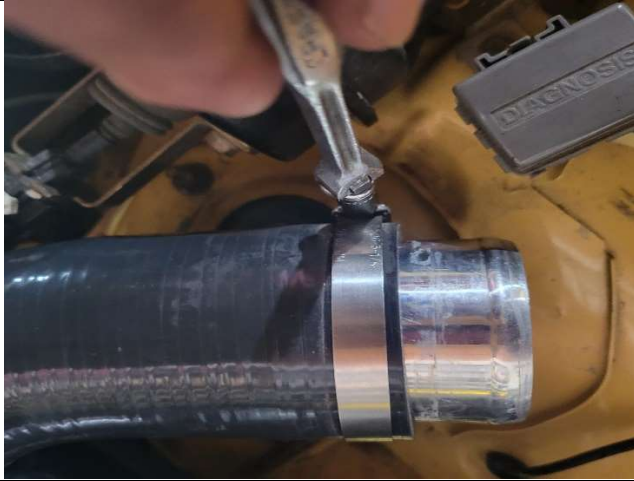
Photo 20-21: Clamp tightened onto pipe insert
