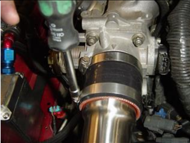
Photo 20-7: Tighten clamp while holding in position
