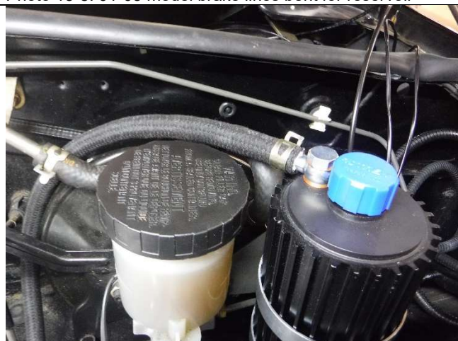
Photo 13-10: Oil cooler to reservoir hose attached
