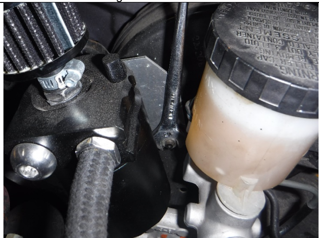
Photo 18-16: Wrench on 12 mm nut
