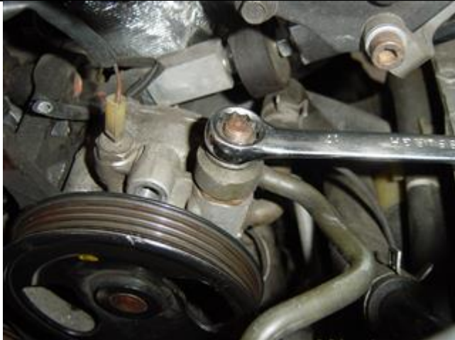
Photo 9-3: Loosen P/S hose and push back
