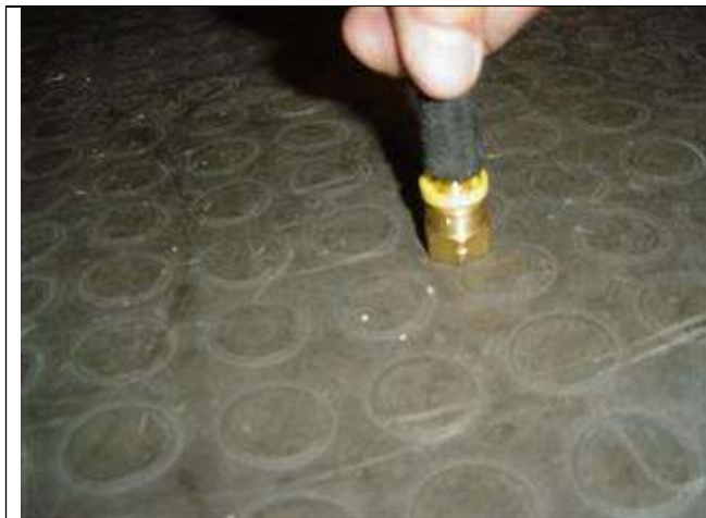
Photo 11-17: Fitting installed on the oil hose
