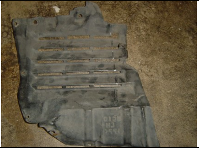
Photo 11-2: Remove inner fender panel
