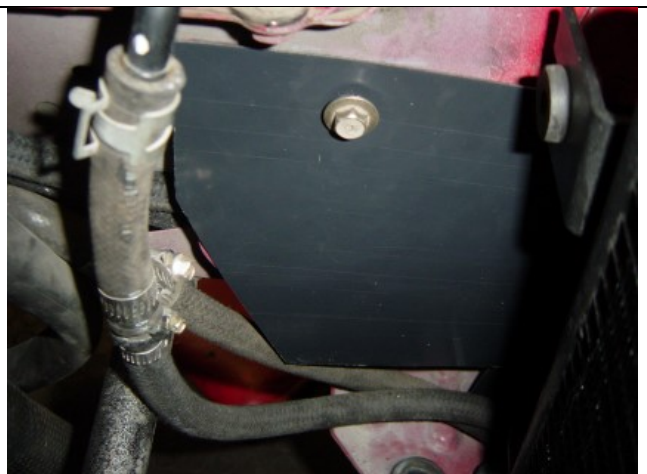
Photo 6-8: Side panel bolted with P/S oil lines
