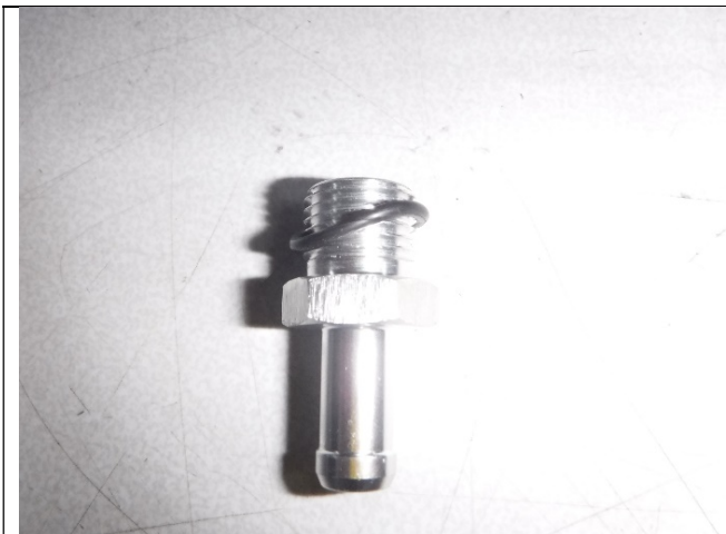
Photo 18-3: 3/8" hose fitting with O-ring
