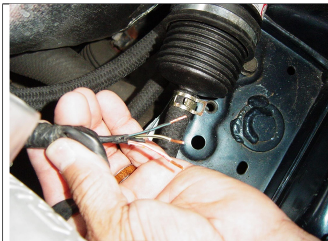
Photo 19-11: ECU side harness wires stripped
