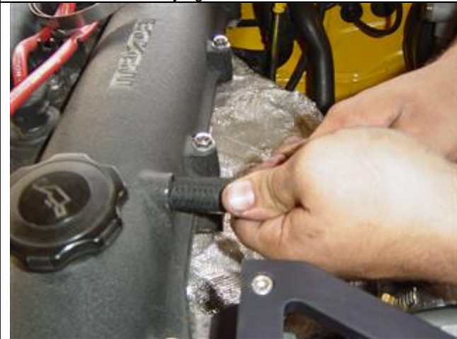
Photo 18-21: Press breather hose onto the valve cover fitting
