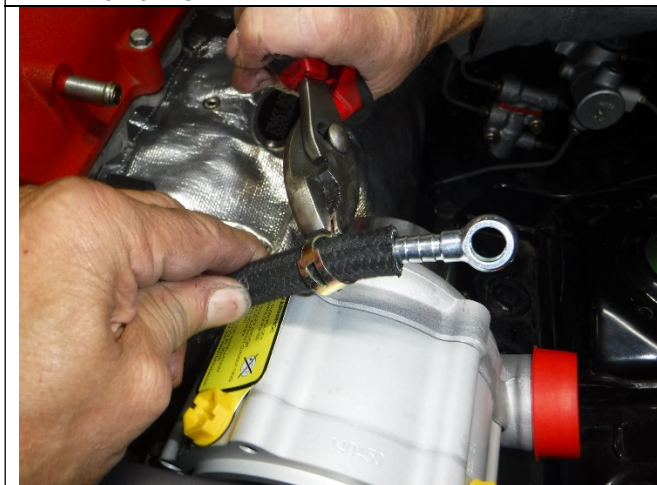
Photo 13-17: Bayonet fitting installed with clamp
