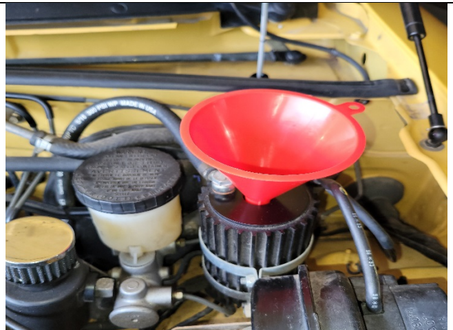
Photo 22-2: Reservoir filled about 3/4 to start
