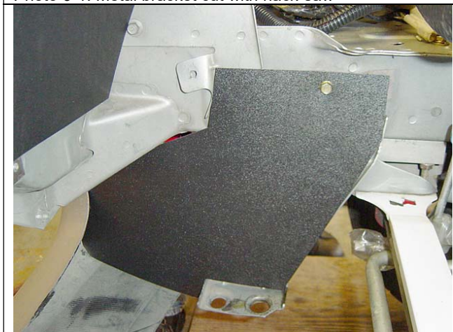
Photo 6-3: Right side plastic panel installed
