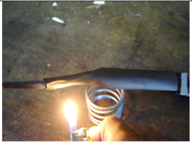
Photo 19-8: Tubing shrunk over harness
