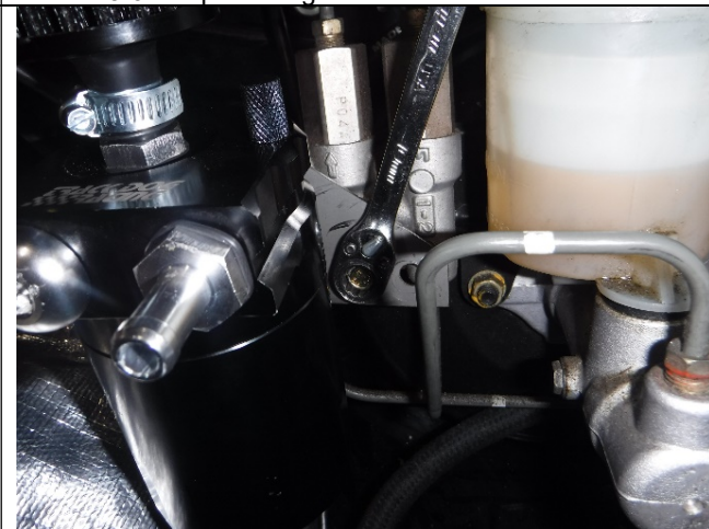
Photo 18-11: Catch can mounted to inside hole
