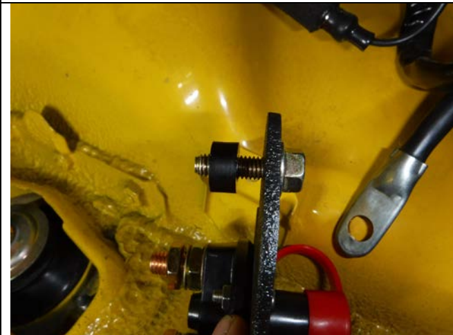
Photo 2-7: Spacer and 25 mm bolt on bracket
