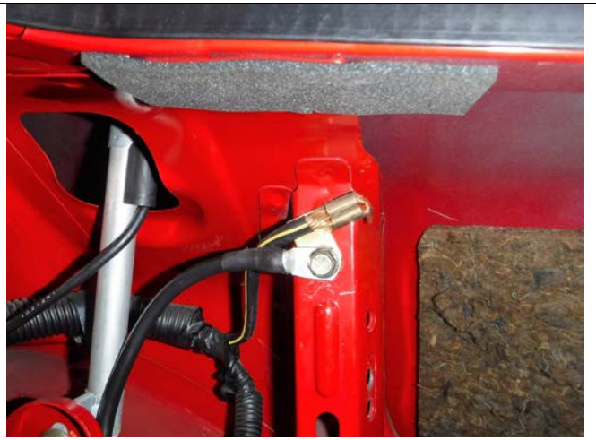
Photo 2-2: Ground strap cut off, new ground strap installed
