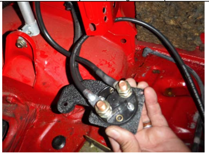
Photo 2-4: Ground strap with post bracket attached
