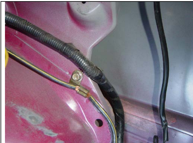
Photo 3-1: Ground strap attached to chassis
