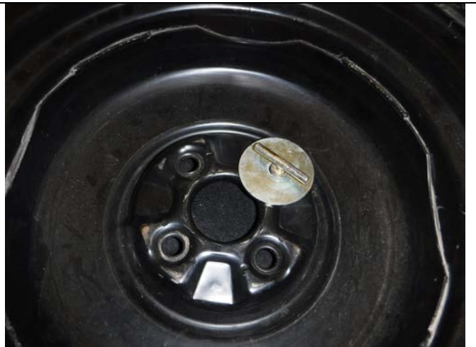
Photo 2-10: Spare tire mounting bolt installed in wheel stud opening
