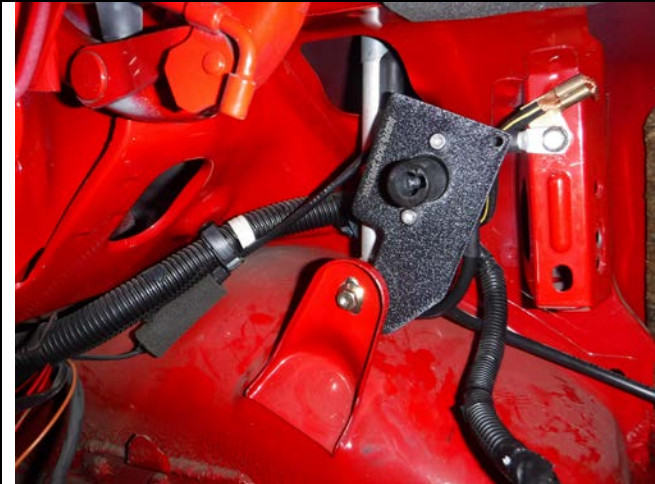
Photo 2-5: Disconnect bracket installed behind bracket
