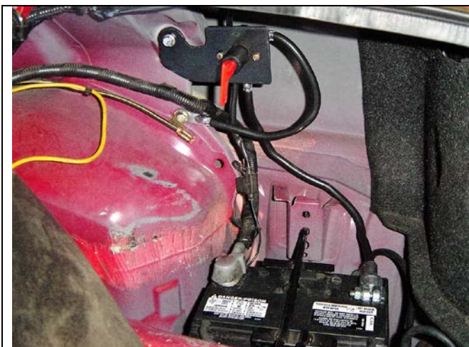
Photo 3-7: Disconnect switch with key
