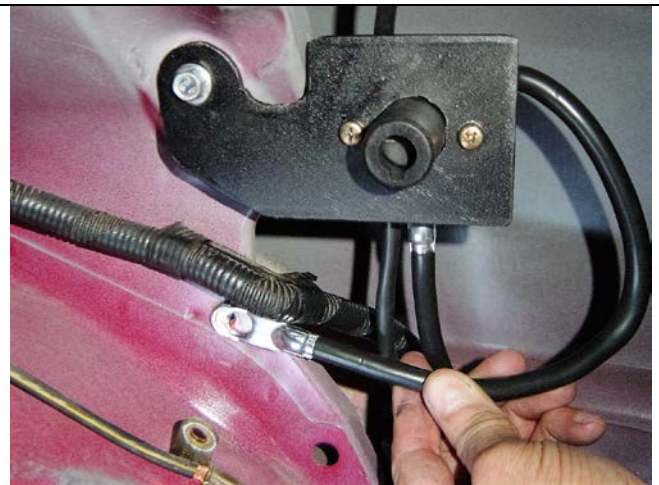
Photo 3-6: Disconnect bracket and ground strap
