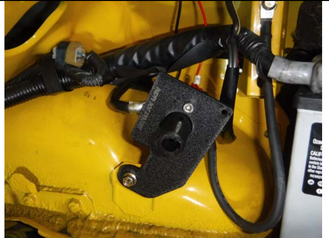
Photo 2-6: Disconnect bracket installed in front of bracket
