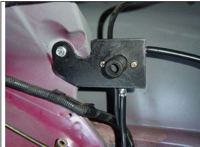
Photo 3-5: Disconnect bracket installed
