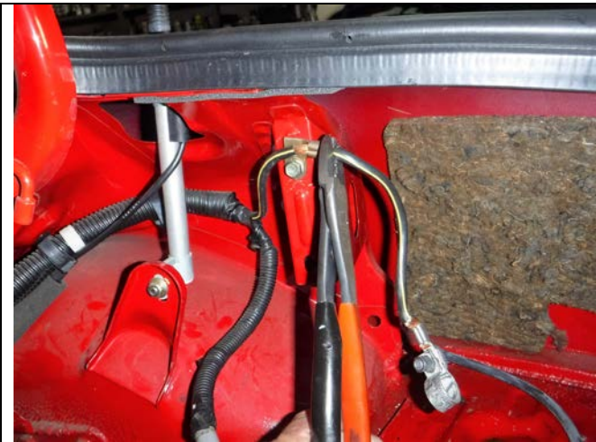
Photo 2-1: Ground strap to be cut
