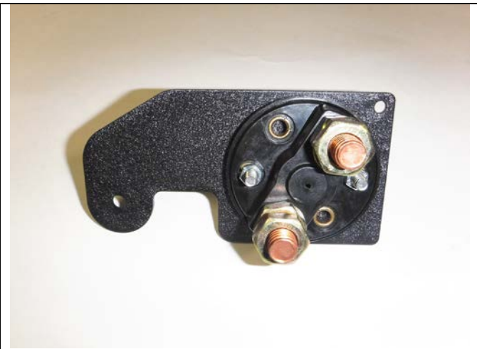
Photo 1-2: Hardware installed on disconnect switch
