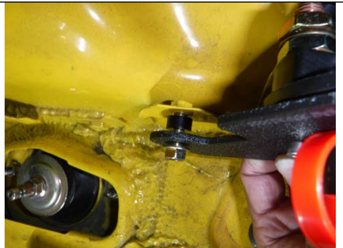
Photo 2-8: Bracket with hardware in fender mount
