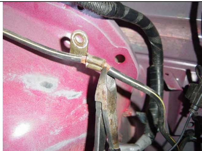
Photo 3-2: Ground strap to battery cut off
