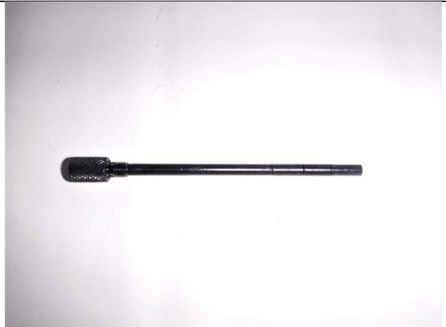
Photo 6-2: Dip stick oil level marks
