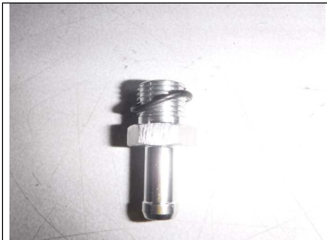
Photo 1-3: 3/8" hose fitting with O-ring
