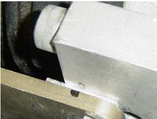
Photo 15: Shim on MP62 supercharger setup
