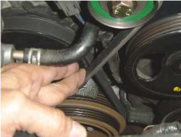
Photo 11: Adjust belt tension to about +/- 1/4" deflection
