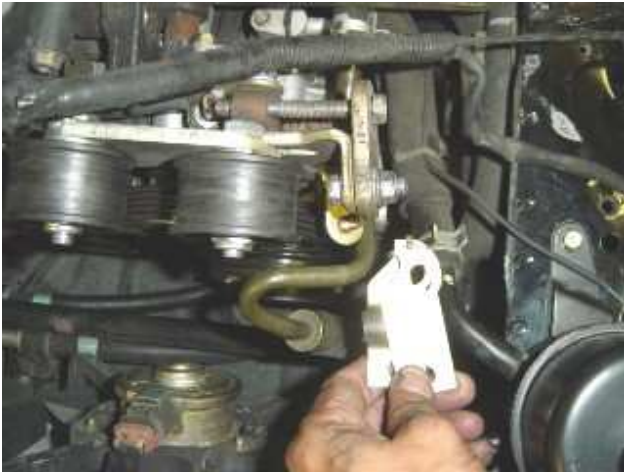
Photo 1: Remove bracket from P/S line
