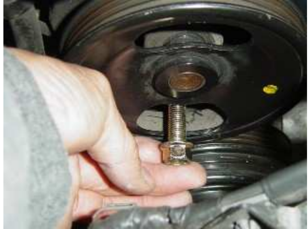
Photo 6: Install the 14 mm bolt through the P/S pulley
