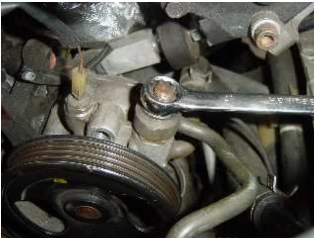
Photo 3: Loosen the P/S line so the hard line can be moved
