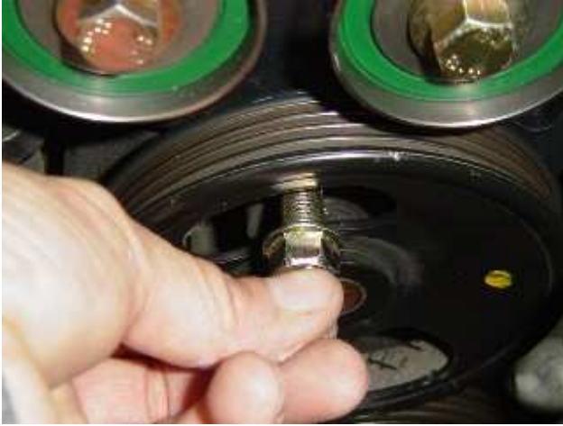
Photo 5: Install the 14 mm bolt through the P/S pulley
