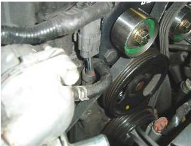
Photo 7: Install belt between the pulleys
