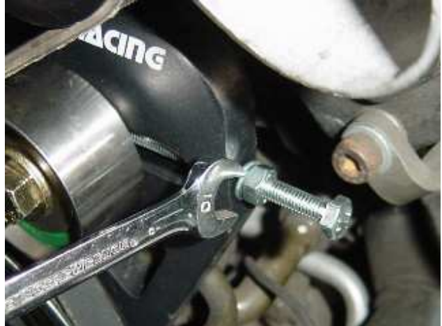
Photo 10: Tighten the Jam Nut when tensioning is complete
