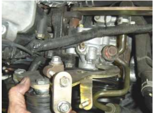
Photo 2: Remove JRSC pulley tensioner system
