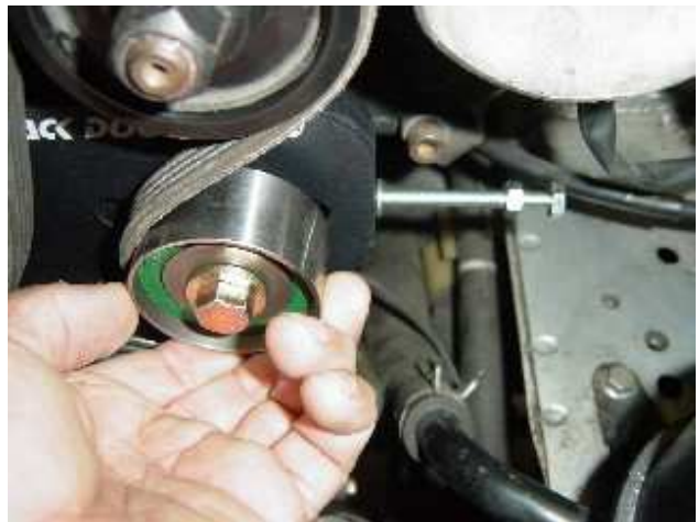
Photo 8: Apply tension to the adjustable pulley while tightening down the tensioner bolt by hand
