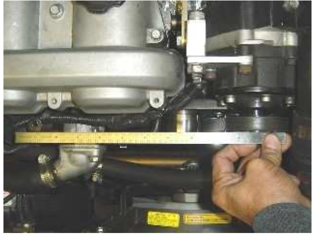
Photo 14: Check for horizontal alignment
