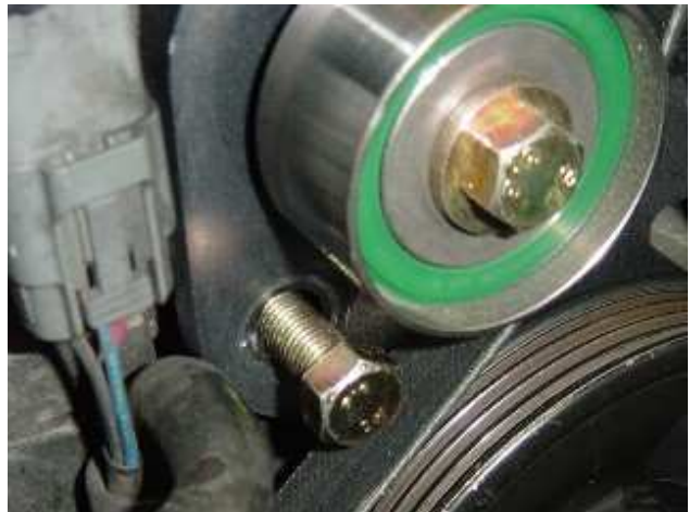
Photo 4: Install the TDR Tensioner Bracket and the 14 mm bolt to hold the assembly in place
