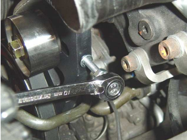
Photo 9: Adjust the belt tension by turning the 10 mm bolt using a ratcheting wrench
