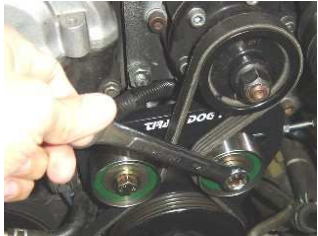
Photo 12: Tighten the 14 mm pulley bolt after tensioning is complete
