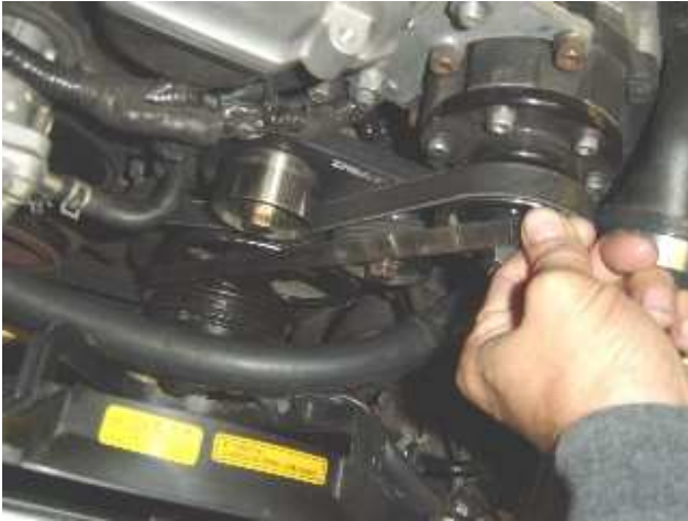
Photo 13: Check for vertical alignment
