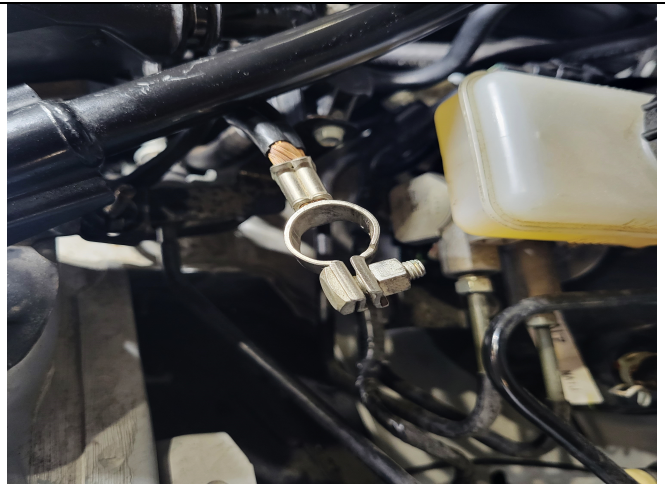
Photo 3-2: Factory ground Post cable at new location
