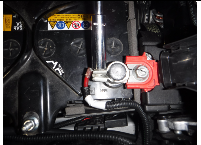
Photo 1-2: Positive battery cable removed from batterypost
