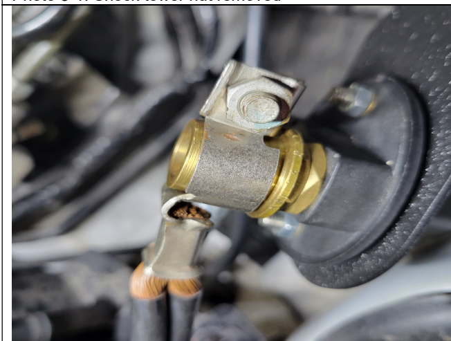
Photo 5-3: Factory cable attaches to the brass post
