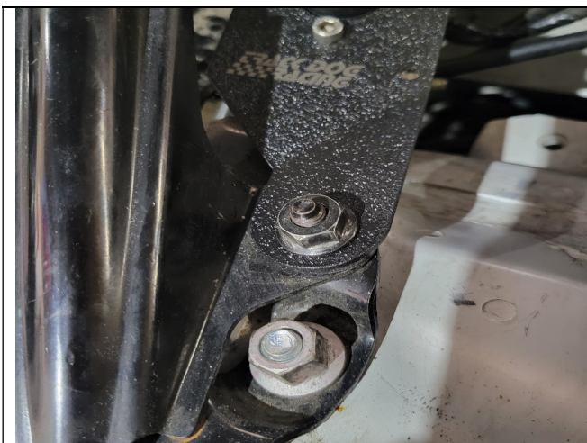
Photo 5-5: Disconnect mounted to shock tower brace
