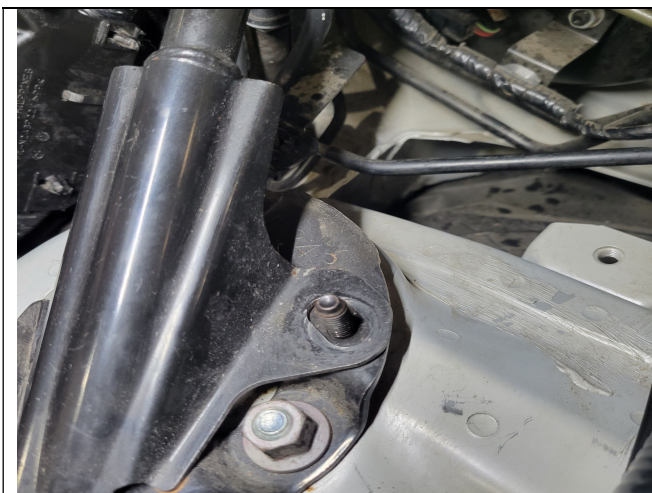
Photo 5-1: Shock tower nut removed
