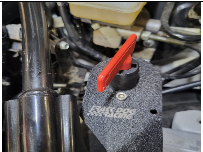
Photo 6-2: Battery ON position
