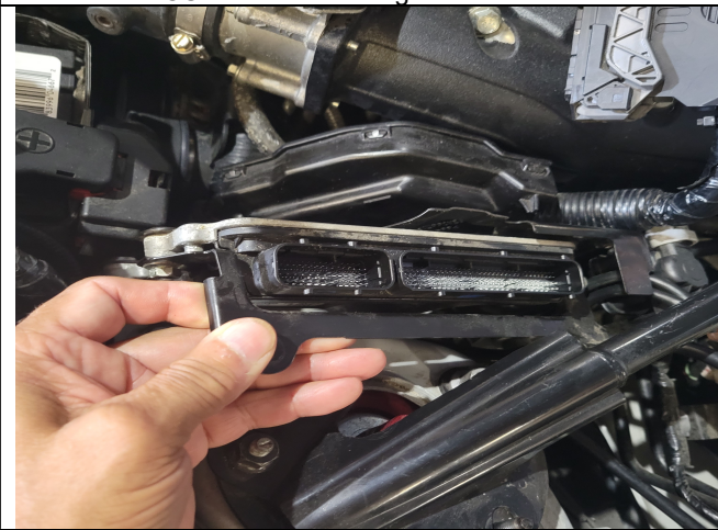
Photo 2-9: Remove ECU from mounting area
