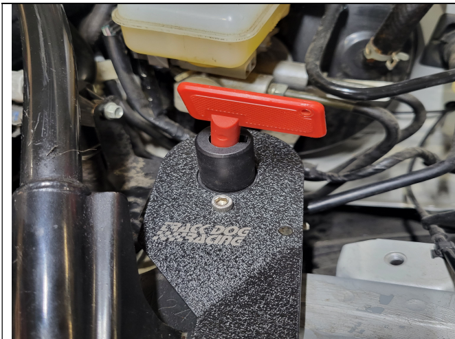
Photo 6-1: Battery OFF position key removal
