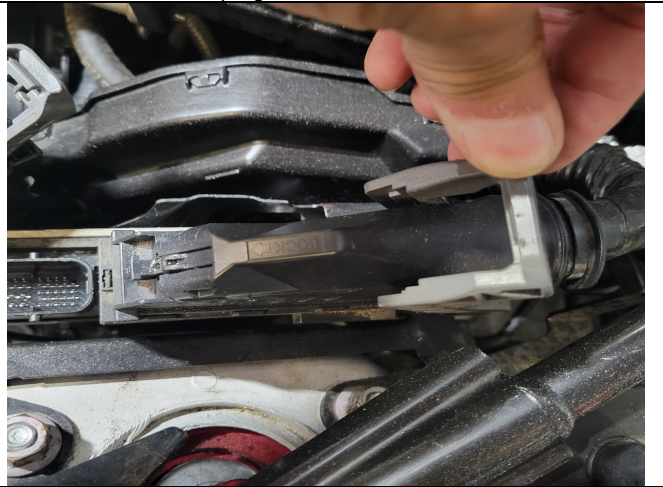
Photo 2-4: Harness plug rotated for removal
