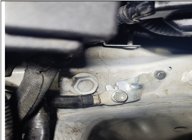
Photo 3-1: Factory chassis ground position
