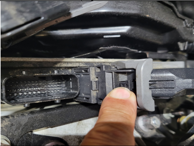
Photo 2-3: ECU harness plug release
