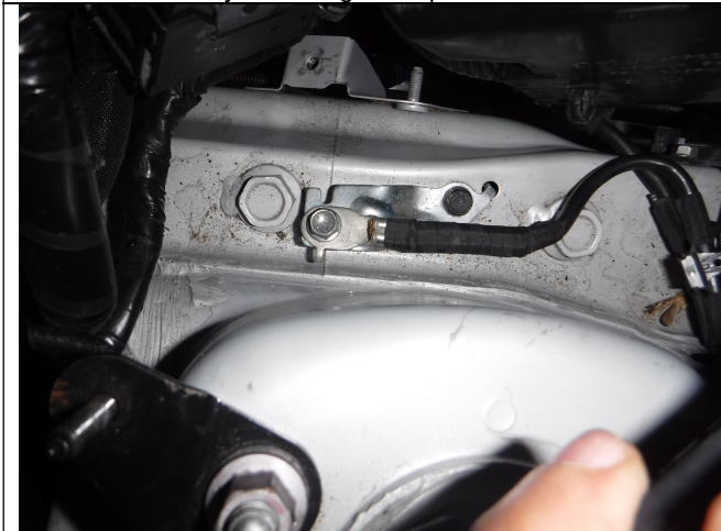
Photo 3-3: Factory chassis ground new position
