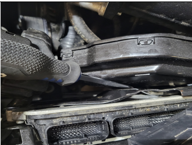
Photo 2-5: Secondary ECU box removed
