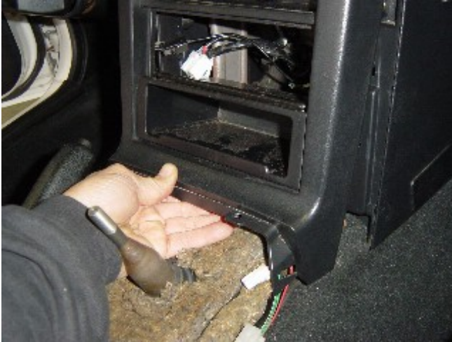
Photo 3-E: Remove the radio wiring
