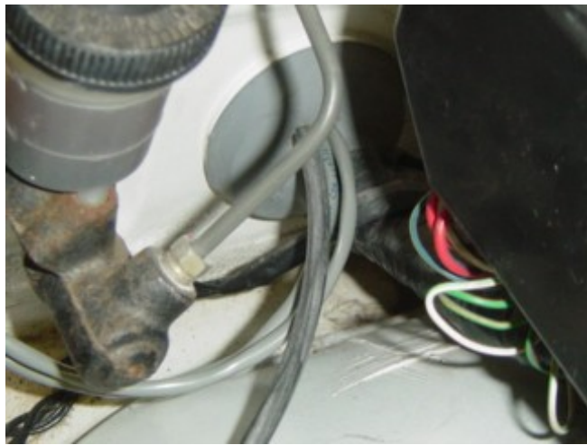
Photo 5-F: Sensor cables and vacuum hose pulled through the firewall wiring boot
