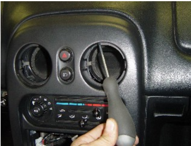
Photo 3-C: Remove the Phillips screw at the top of the air vent on the right side
