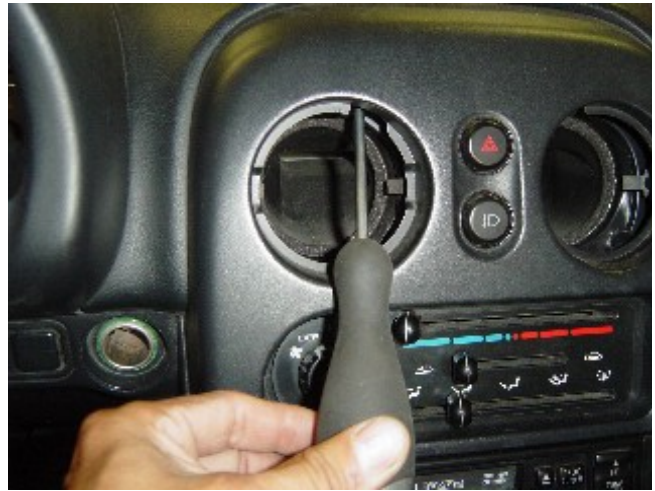
Photo 3-D: Remove the Phillips screw at the top of the air vent on the left side
