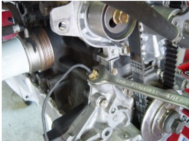
Photo 9-D: Oil temperature can be from a remote oil filter kit or by replacing the plug in the oil pump
