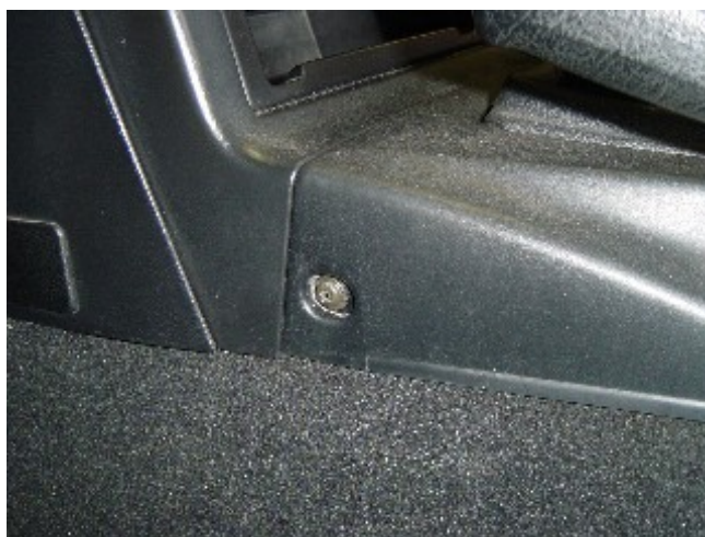
Photo 1-D: Remove the Phillip screws from each side of the console
