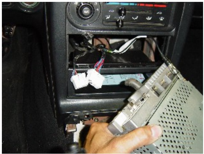
Photo 2-D: Remove wiring and slide radio out
