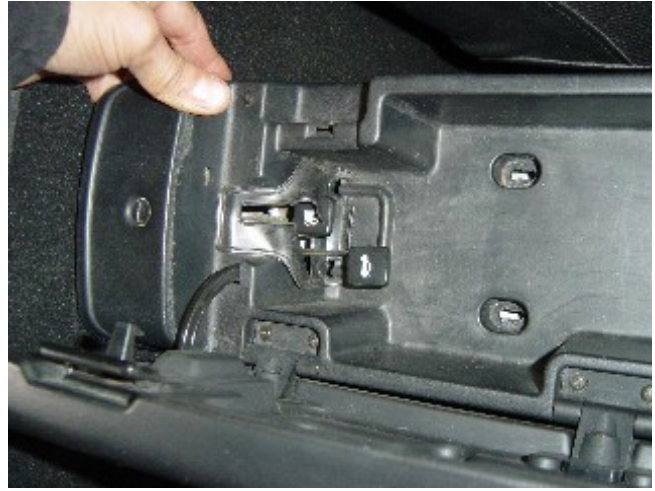
Photo 1-F: Pull the console forward to clear the levers
