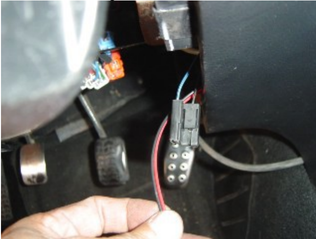
Photo 6-A: Pull the cigarette lighter connector to the side for access for wiring
