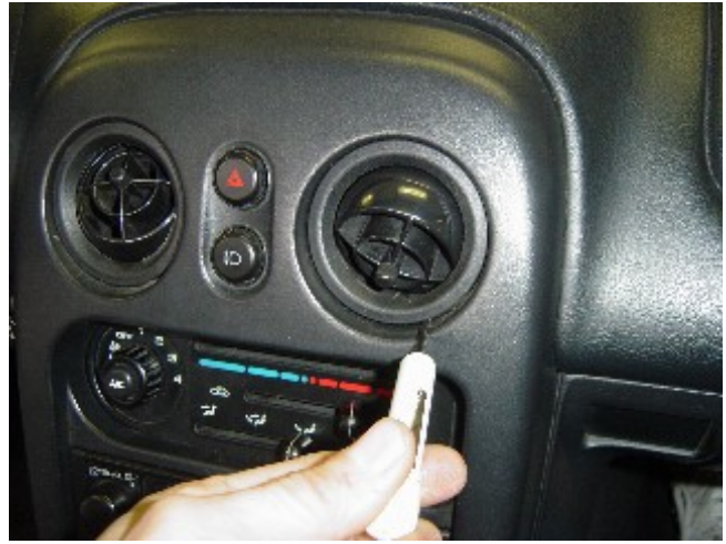
Photo 3-B: Remove the vent ring with a small screwdriver
