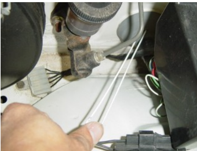
Photo 5-C: Bend a coat hanger and push into the cut
