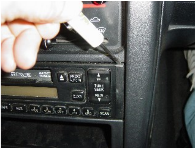
Photo 2-A: Remove the radio covers on each side with a small screwdriver
