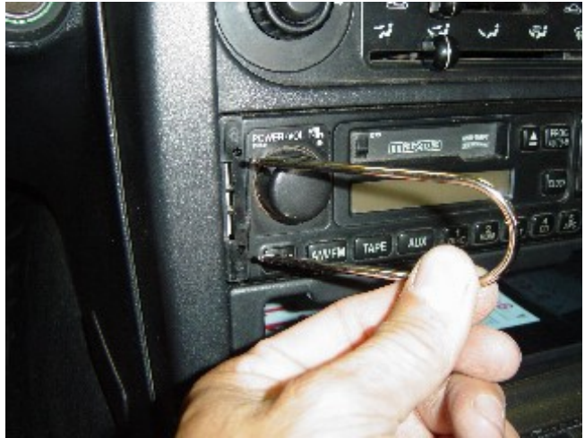
Photo 2-B: Insert the radio removal tool on each side through the exposed holes
