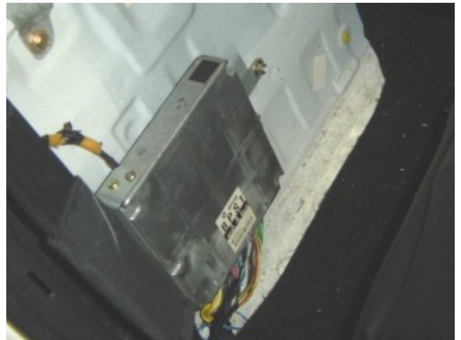
Photo 7-D: ECU on the back wall behind the seat
