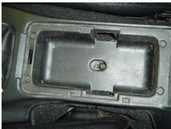
Photo 1-C: Remove the Phillip screw from cup holder
