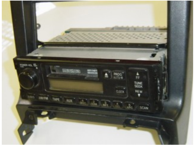
Photo 4-B: Insert the radio into the lower section of the bezel until the clips are secure in the bezel
