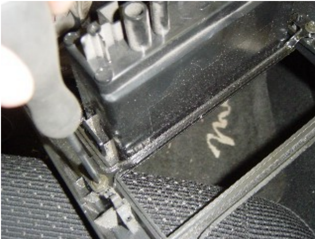
Photo 4-A: Remove the Phillip screws from the storage bin and remove
