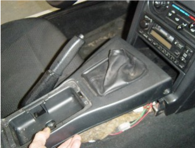
Photo 1-E: Lift the console upwards over the shift knob
