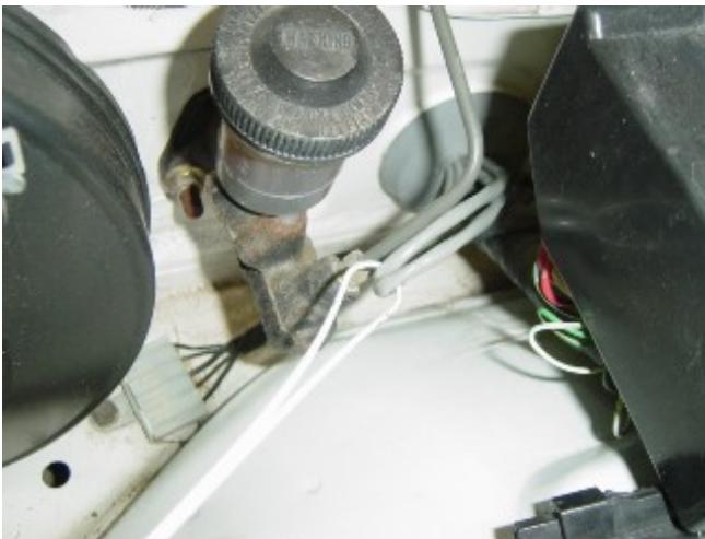
Photo 5-E: Pull the coat hanger out along with the Sensor cables
