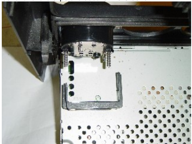
Photo 4-D: Modify the gauge mounting bracket to hold the gauge panel to the bezel
