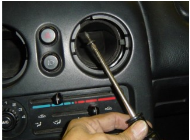
Photo 8-B: Take caution when installing these two screws, as they are a little difficult to start
