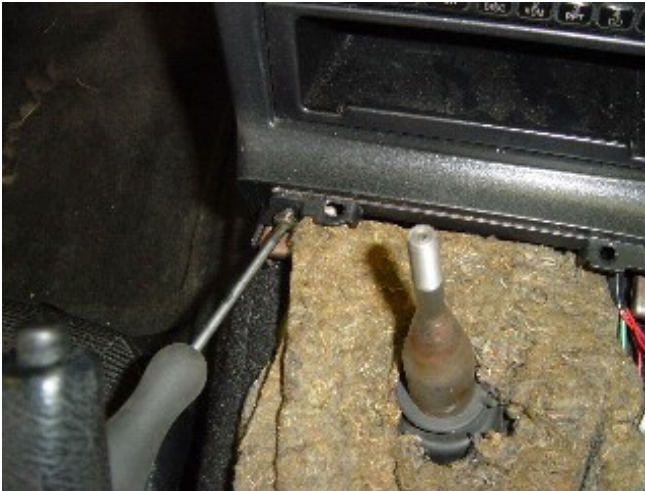
Photo 3-A: Remove the lower Phillips screw on the lower left side
