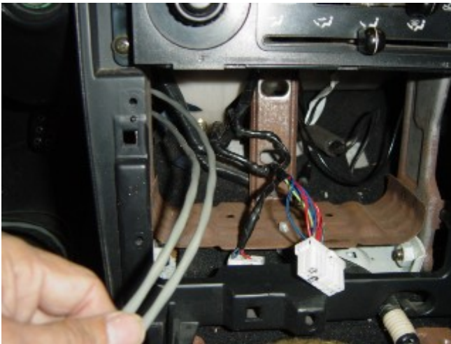
Photo 5-A: Feed the sensor wires through the radio opening and toward the firewall
