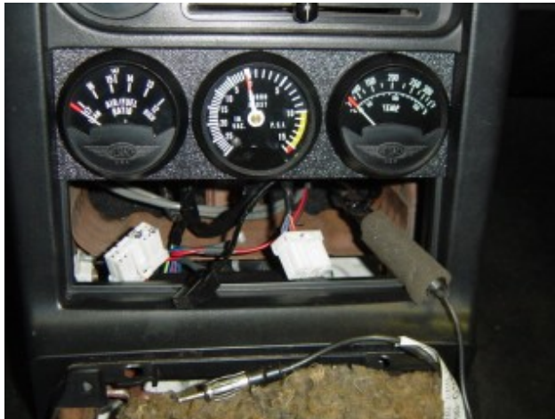
Photo 8-A: Install bezel and place wiring up front for radio installation
