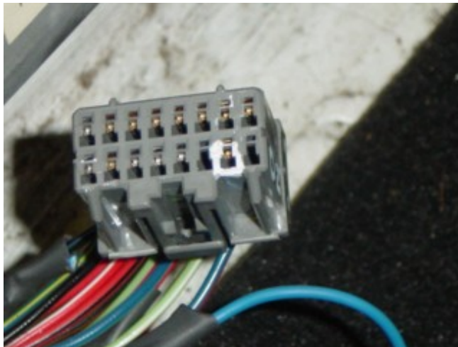
Photo 7-C: O2 Sensor terminal block uses a RED with GREEN TRACER that is second from the end
