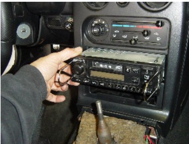
Photo 2-C: Push removal tools toward the outside
