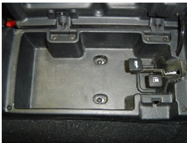
Photo 1-B: Remove the Phillip screws from console
