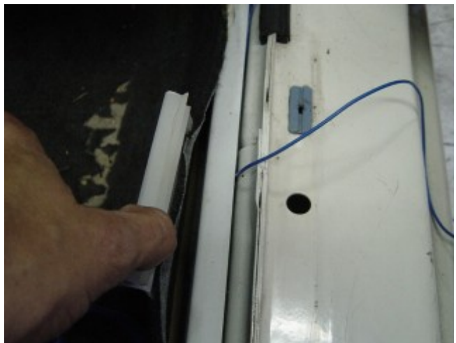
Photo 7-B: O2 Sensor wire traced through the side sill after removing the side sill cover
