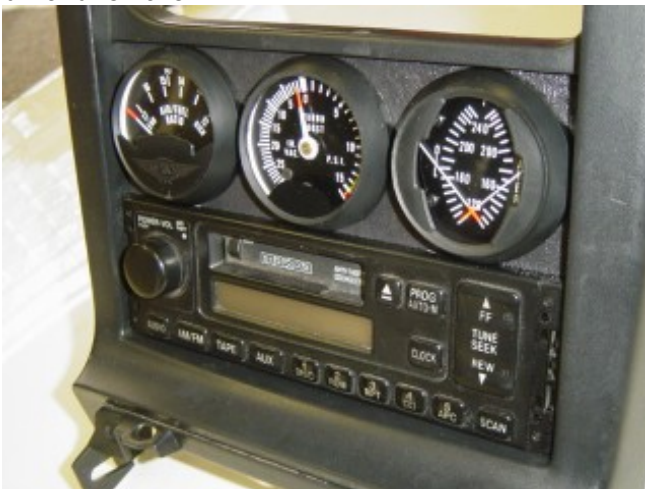
Photo 4-C: Insert one or more of the outside gauges
