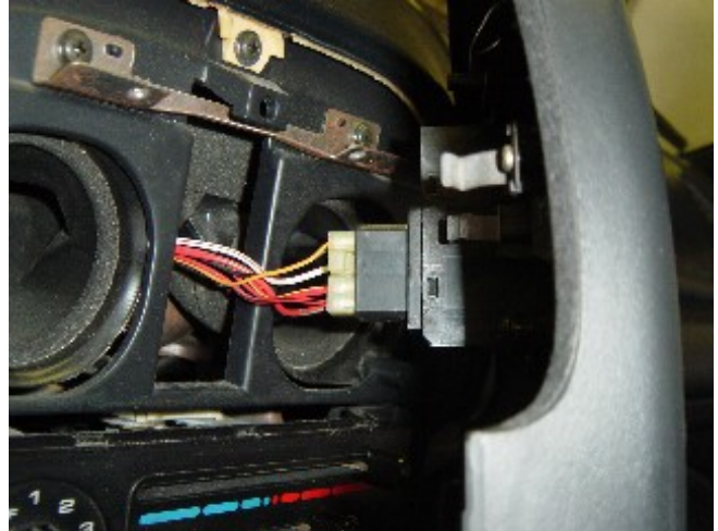
Photo 3-F: Remove the radio wiring
