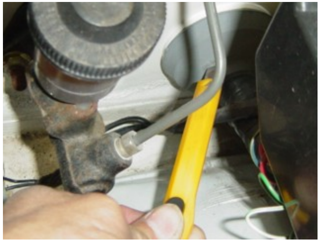
Photo 5-B: Using a knife, cut a slit in the firewall wiring boot
