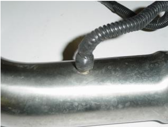
Photo 9-C: Air temperature sensor can be installed using a 1/8" NPT taped hole in the intercooler pipe
