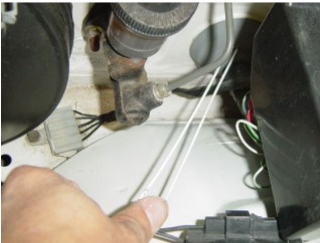
Photo 4-C: Bend a coat hanger and push into the cut
