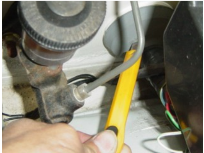
Photo 4-B: Using a knife, cut a slit in the firewall wiring boot
