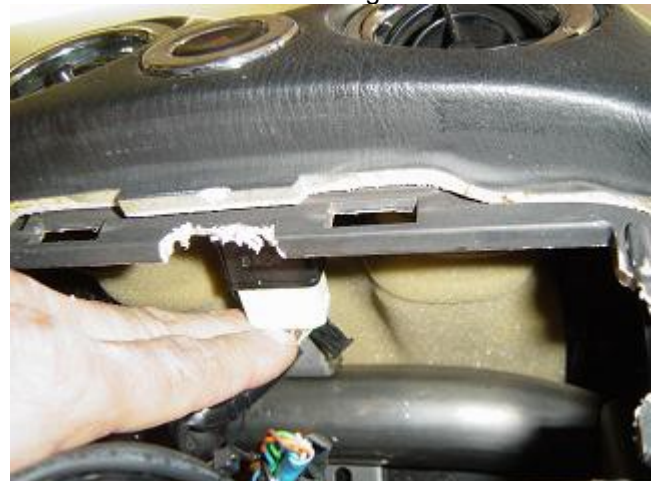
Photo 3-D: Remove hazard warning light connector
