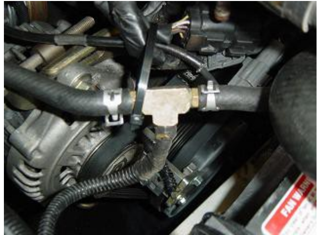
Photo 7-B: Water temperature comes from the Tee provided into the 5/16" hose
