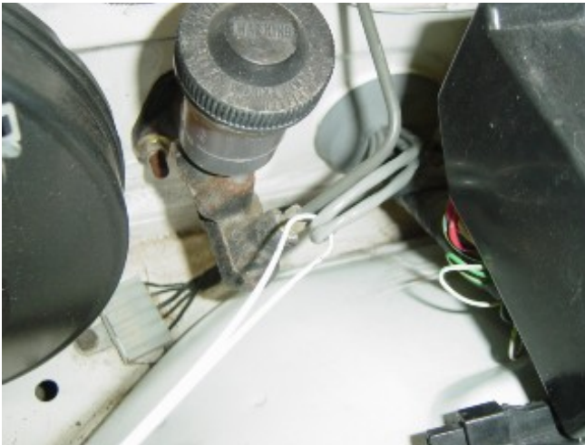
Photo 4-E: Pull the coat hanger out along with the Sensor cables
