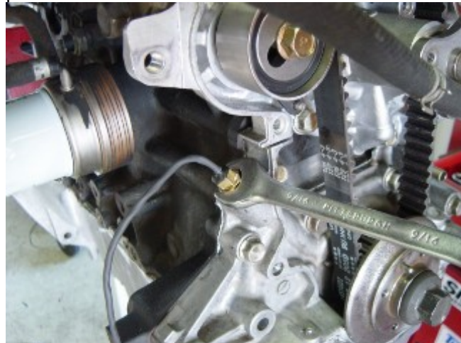
Photo 7-D: Oil temperature can be from a remote oil filter kit or by replacing the plug in the oil pump
