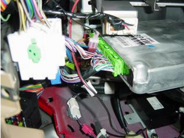
Photo 6-A: Oxygen sensor connection at the ECU
