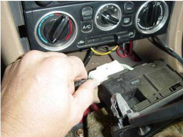
Photo 2-C: Remove the wiring connections from the air bag and cigarette lighter
