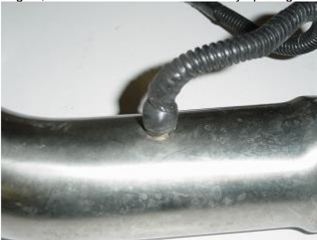
Photo 7-C: Air temperature sensor can be installed using a 1/8" NPT taped hole in the intercooler pipe
