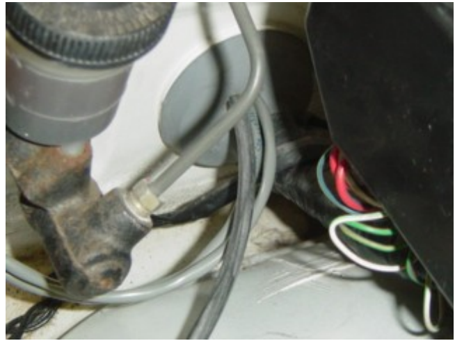
Photo 4-F: Sensor cables and vacuum hose pulled through the firewall wiring boot
