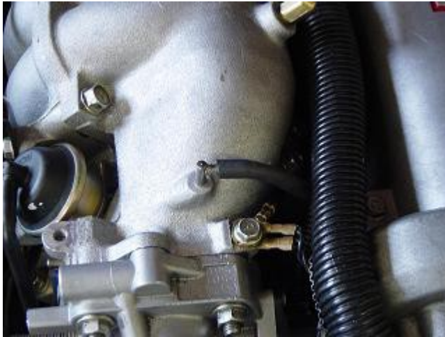
Photo 7-A: Vacuum fitting can be anywhere on the engine, but best nearest the throttle body opening
