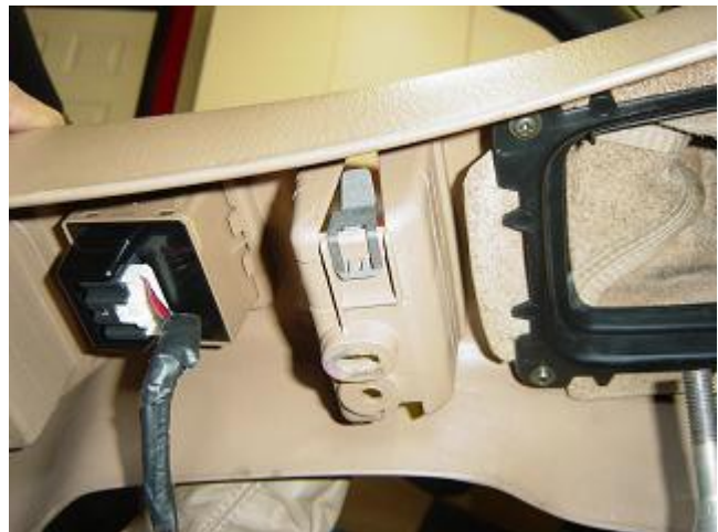
Photo 1-D: Remove light switch connection under the console
