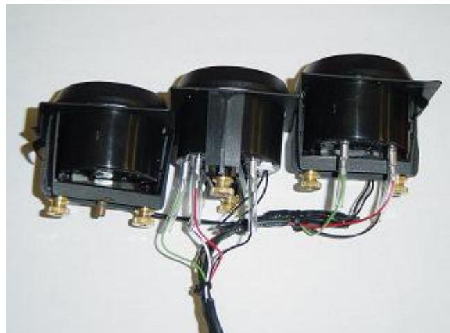
Photo 4-B: Bundle the wires using tie-wraps
