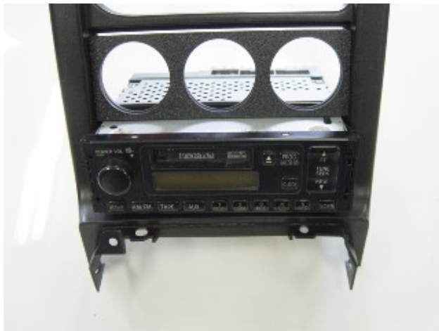
Photo 1-A: Radio and gauge panel mounted into bezel
