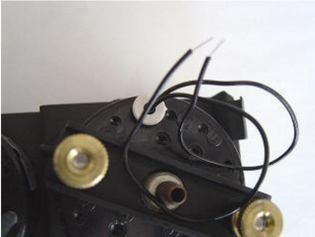
Photo 3-E: Install light into the back of the gauge
