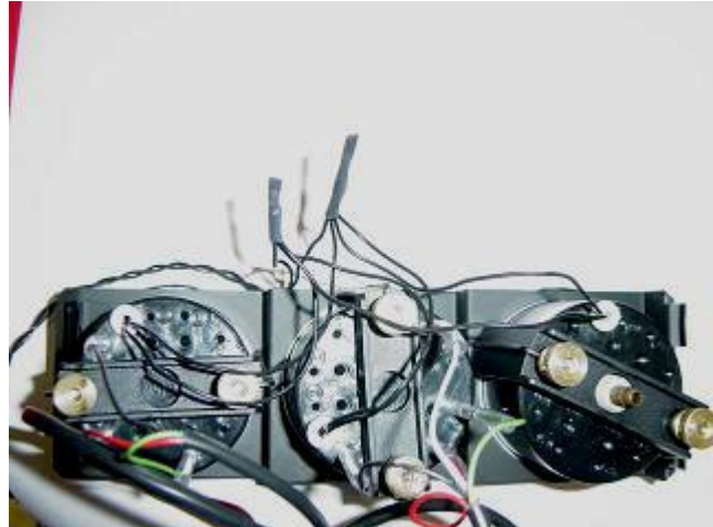
Photo 3-F: Attach the power leads together
