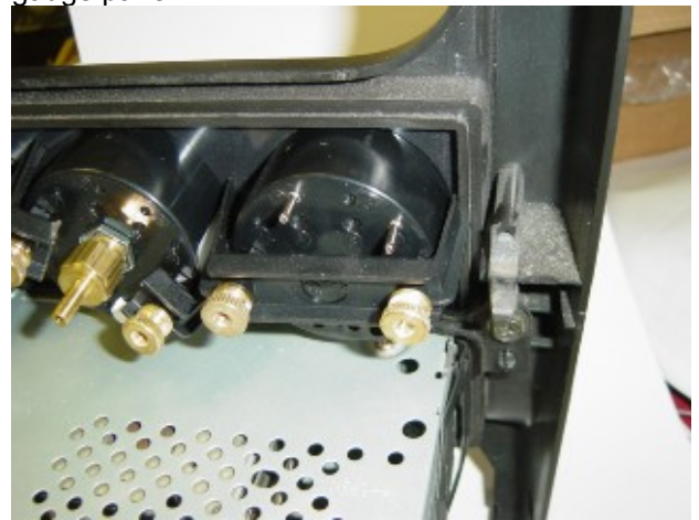
Photo 1-D: Modified mounting bracket installed pressing against bezel
