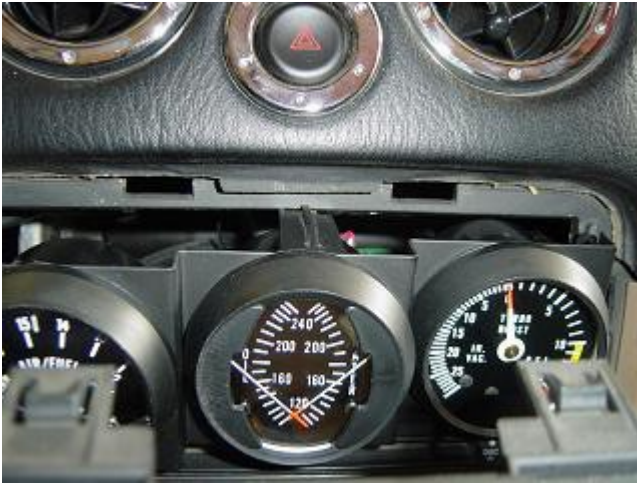
Photo 2-C: Modify dash as required for gauge clearances
