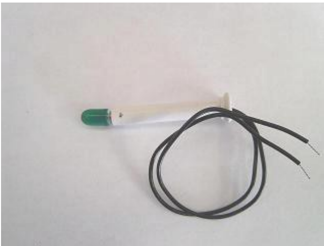
Photo 3-C: Gently install the green rubber cover over the light bulb
