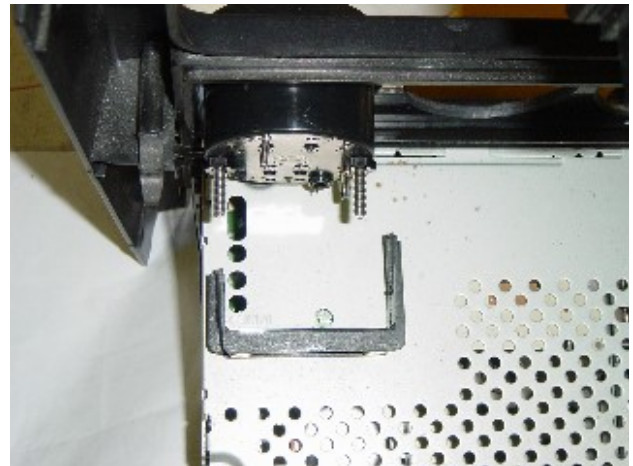
Photo 1-B: Modified mounting bracket to secure gauge panel
