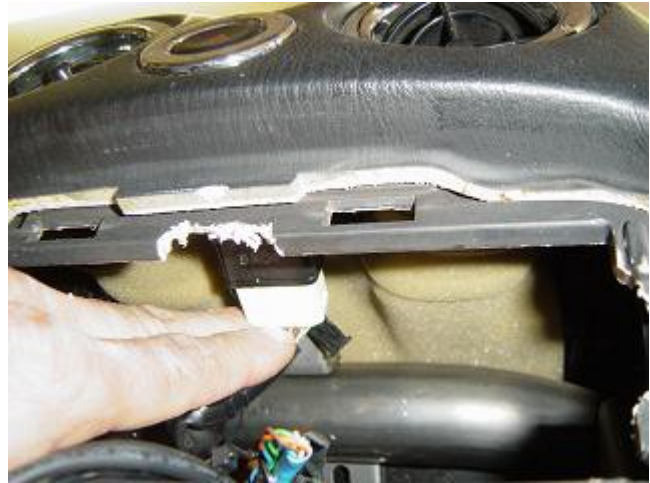
Photo 2-D: Disconnect hazard warning light connector
