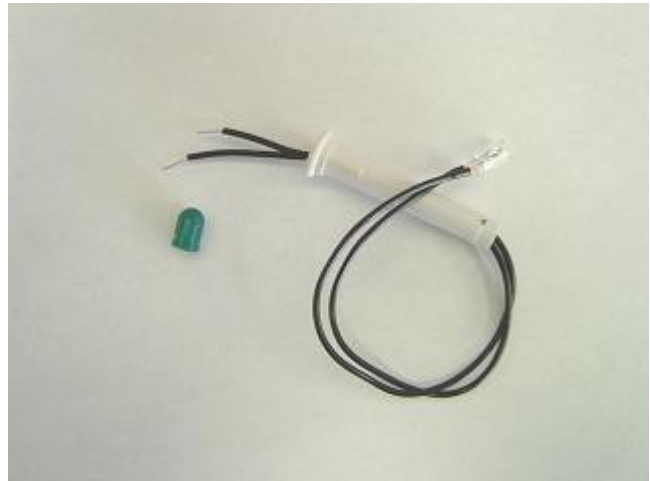
Photo 3-B: Insert the light wiring through the tube opposite of the flange end
