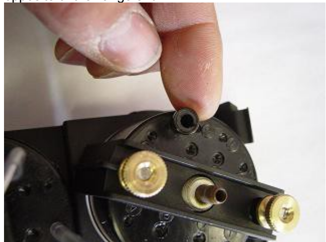
Photo 3-D: Remove the blank plug from the back of the gauge
