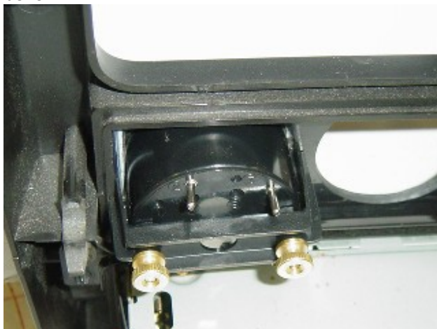
Photo 1-C: Modified mounting bracket installed pressing against bezel
