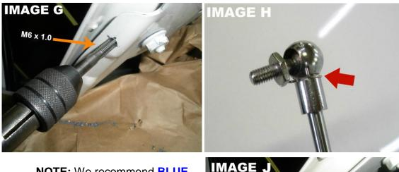
NOTE: We recommend BLUE medium strength thread lock (not included) on the shorter 7/16" (12mm) length ball stud and tighten snug. (IMAGE J) Be careful not to tighten too much or you can strip the threads you just made with the tap. The thread lock will keep it secure.
