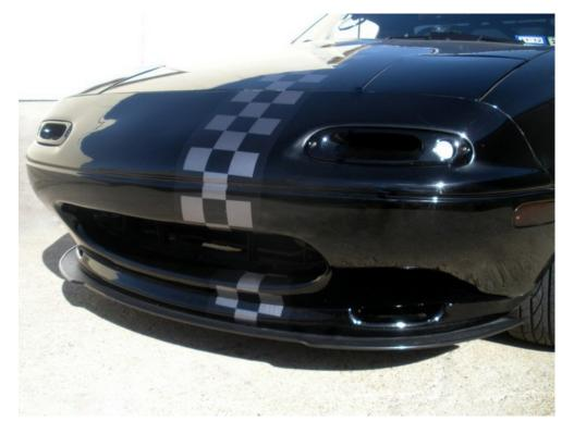
Thank you for purchasing the Track Dog Racing Air Splitter/Protector. The Air Splitter is designed to help protect the factory R-Package lip by allowing the Air Splitter to slide over obstacles, such as steep driveways. The TDR Air Splitter is made from 3/16" thick, high-impact ABS plastic and will surprisingly take a lot of abuse. The textured top finish blends in well with any color however; you might consider painting the R Spoiler for a nicer appearance such as the picture above.
