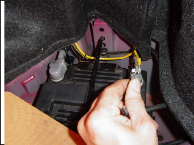
Photo 1-1: Disconnect battery ground
