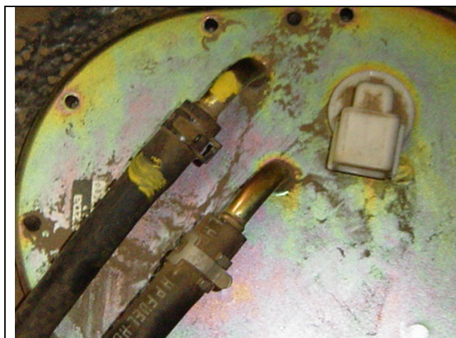
Photo 3-1: Fuel hose marked for reinstallation
