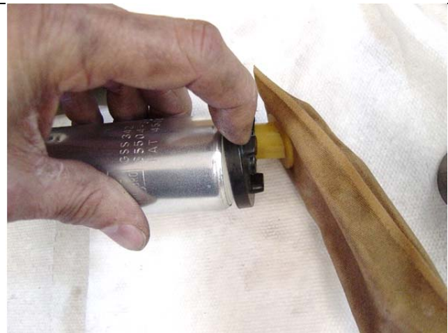
Photo 5-8: Rubber mount on bottom of pump
