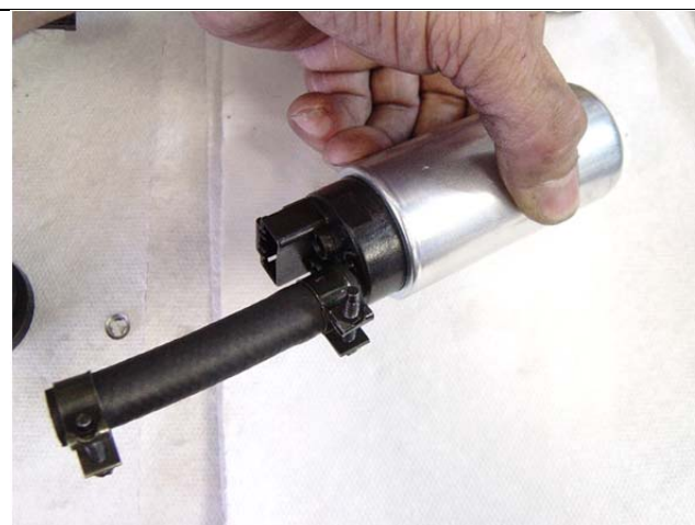
Photo 5-6: New hose installed on fuel pump
