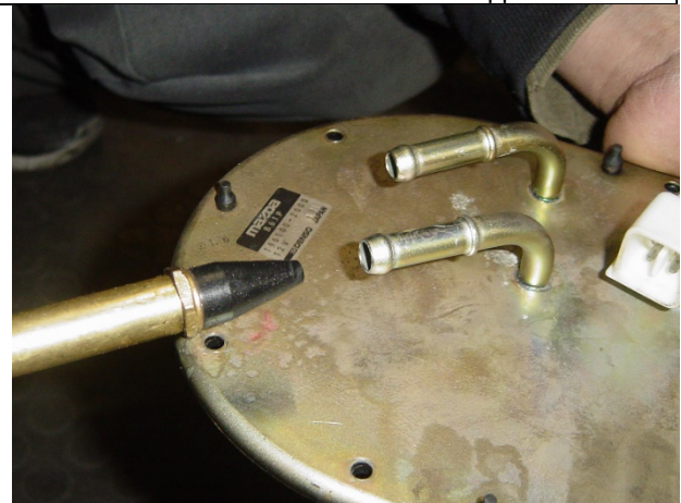
Photo 4-10: Air blown thru inlet tube to clear debris
