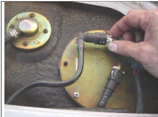
Photo 3-5: Fuel line released
