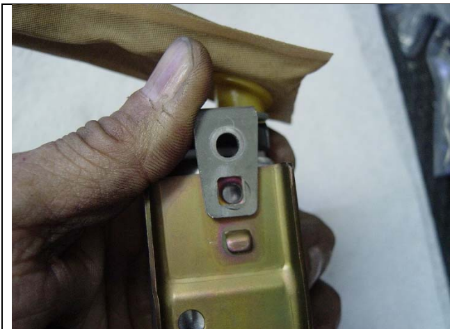
Photo 5-9: L-bracket mounted with screw in square hole
