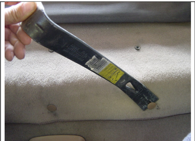
Photo 1-4: Disconnect tabs from carpet deck
