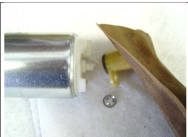
Photo 5-5: Remove strainer clip using a small screwdriver
