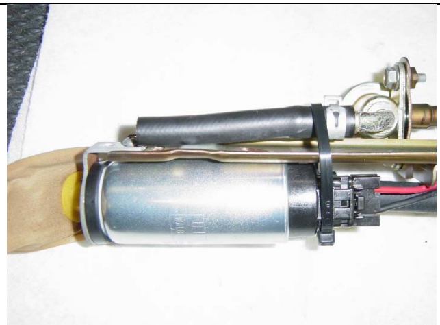
Photo 5-10: Fuel Pump assembly complete
