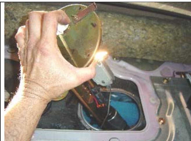
Photo 5-1: Fuel pump assembly being removed
