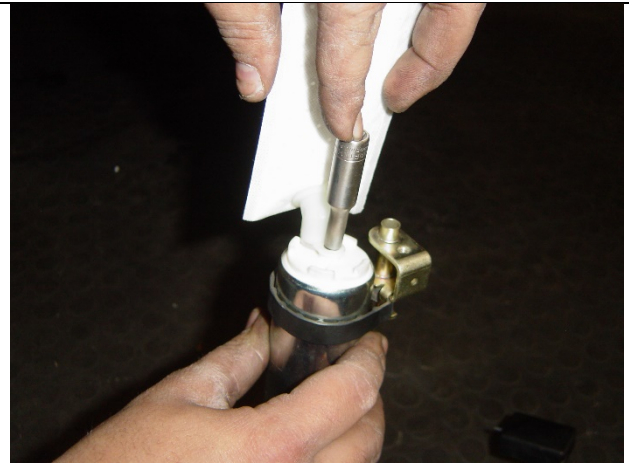
Photo 4-12: Strainer clip installed
