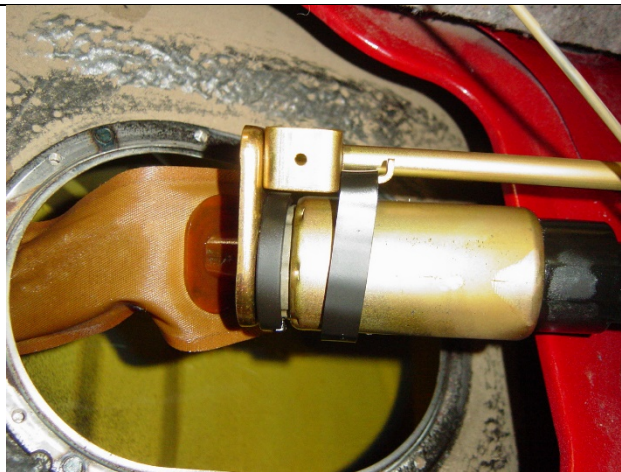
Photo 3-4: Fuel pump pulled from tank
