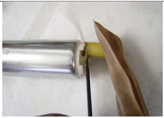
Photo 4-2: Strainer clip removed
