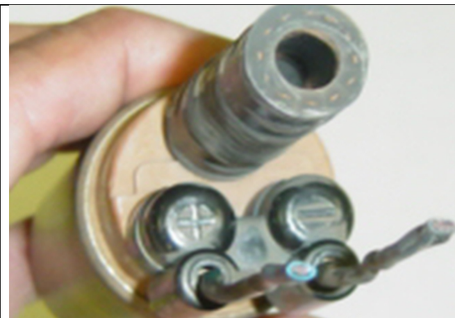
Photo 2-1: Screw type fuel pump termination
