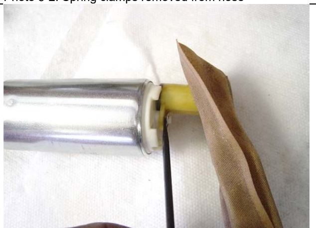
Photo 5-4: Strainer clip removed with small screw driver
