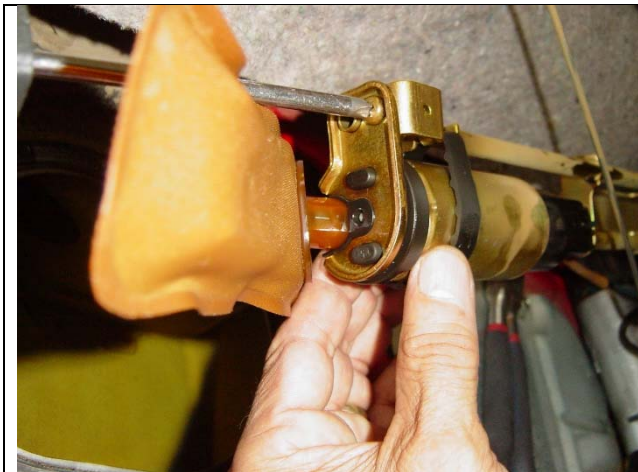
Photo 4-1: Base removed from pump
