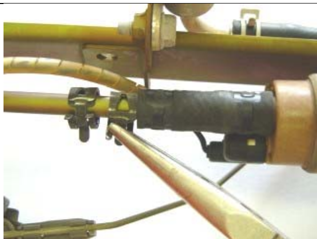
Photo 5-2: Spring clamps removed from hose
