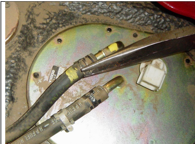
Photo 3-3: Remove spring clamps and harness
