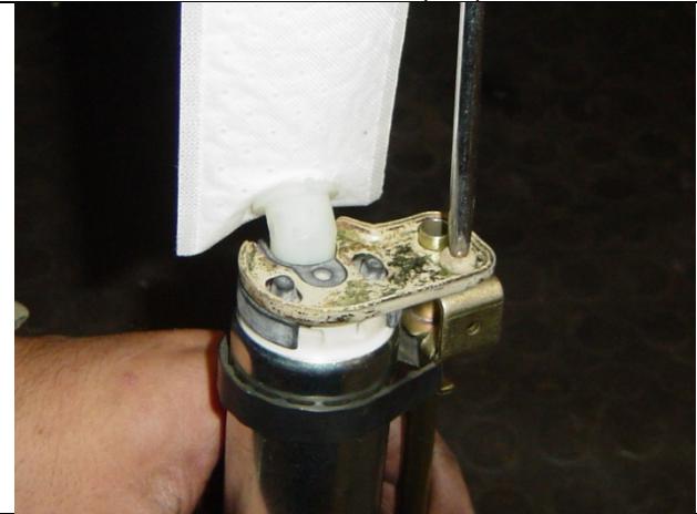
Photo 4-13: Bottom mounting bracket installed
