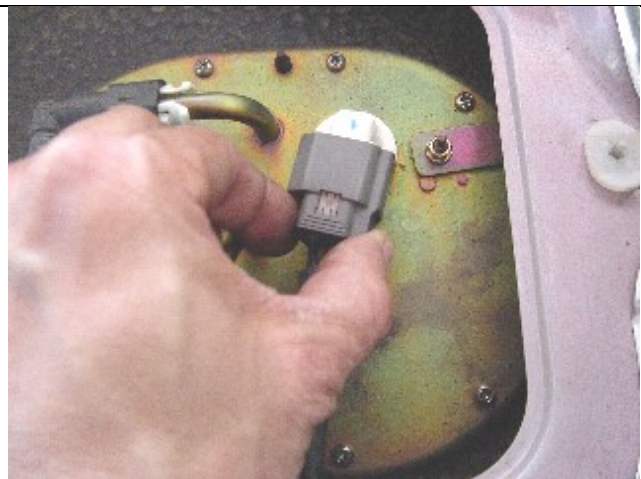
Photo 3-6: Releases electrical connection
