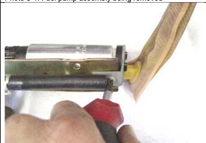
Photo 5-3: Bottom mount screw removed
