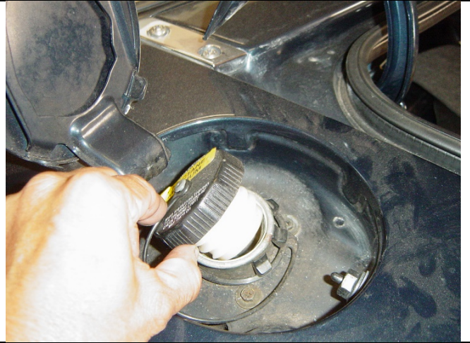
Photo 1-2: Remove gas cap to relieve pressure
