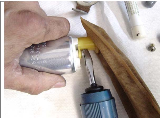
Photo 5-7: Clip installed on strainer
