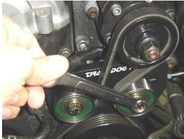
Photo 14: Tighten the 14 mm pulley bolt after tensioning is complete
