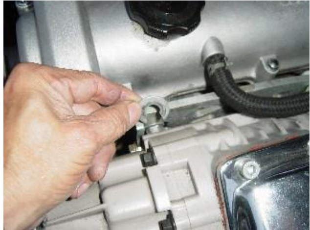
Photo 18: Shim on M45 supercharger setup
