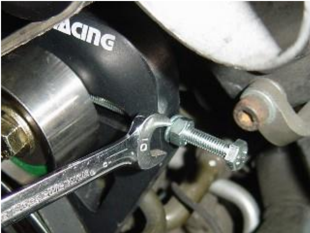
Photo 13: Tighten the Jam Nut when tensioning is complete
