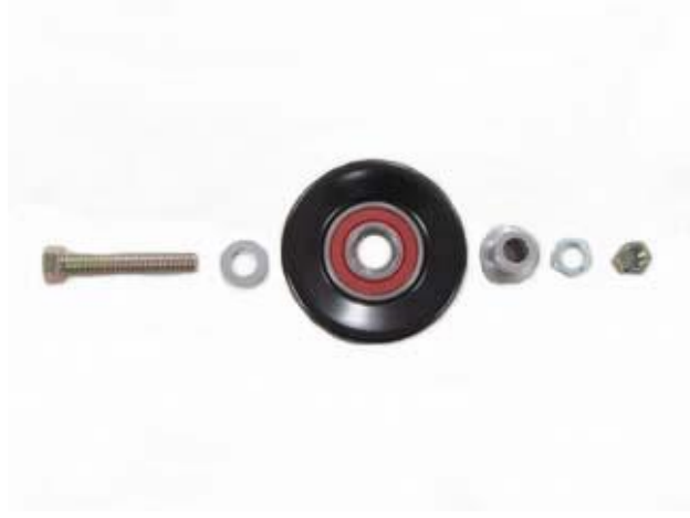
Photo 8: OPTIONAL A/C Delete Pulley necessary to extend the length of the belt path: Note the use of a special spacer/adaptor
