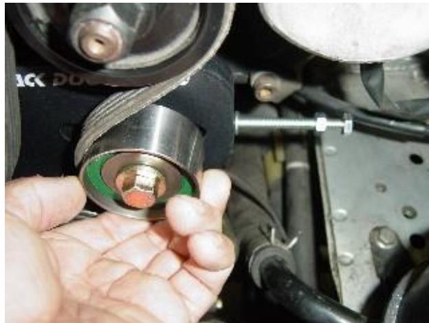
Photo 10: Apply tension to the adjustable pulley while tightening down the tensioner bolt by hand
