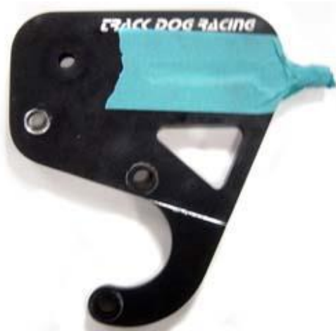
Photo 6: OPTIONAL: Tape up the bracket to protect the adjustment groove from shavings and mark it
