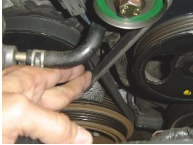
Photo 12: Adjust belt tension to about +/- 1/4" deflection
