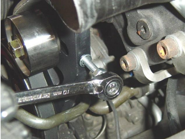
Photo 11: Adjust the belt tension by turning the 10 mm bolt using a ratcheting wrench
