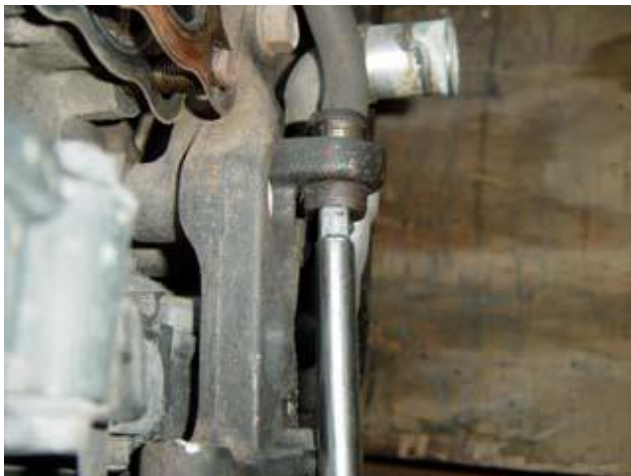
Photo 1: Hammer the spacer back
