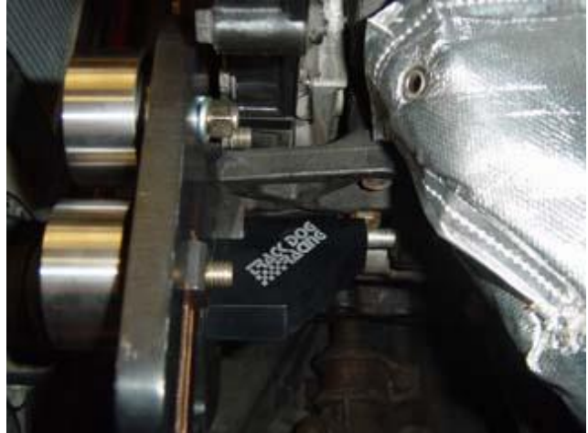
Photo 4: Install long P/S bolt through TDR Power Steering Delete Bracket.
