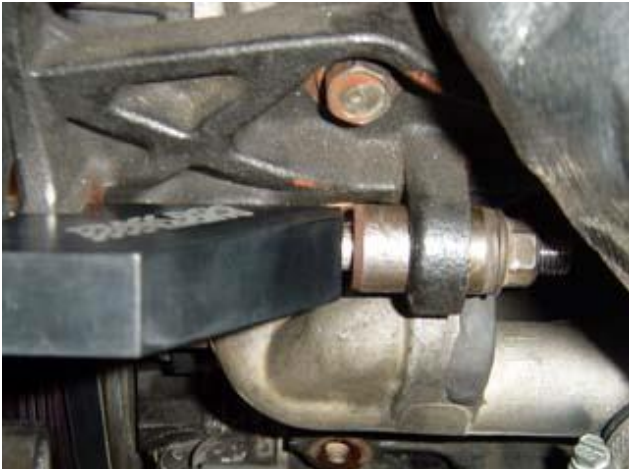
Photo 5: Tighten the 14 mm long bolt to bring spacer back forward.
