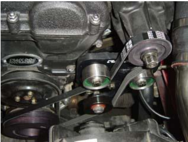
Photo 9: OPTIONAL A/C Delete Pulley: Note the belt path.
