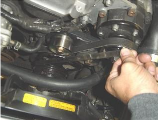
Photo 15: Check for vertical alignment
