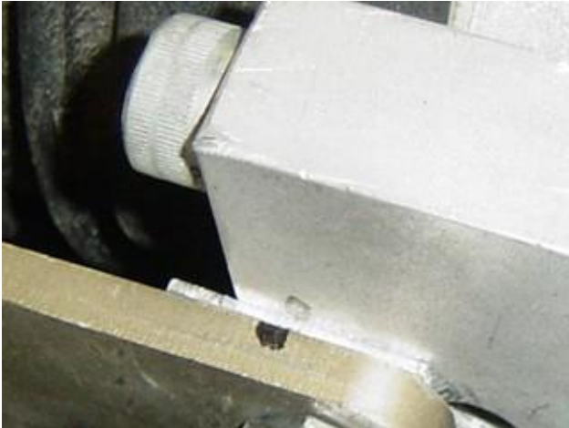
Photo 17: Shim on MP62 supercharger setup
