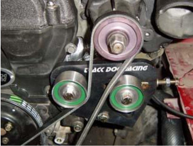
Photo 7: OPTIONAL: Cut the aluminum TDR tensioner for a slightly cleaner look on cars with A/C.
