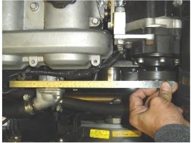
Photo 16: Check for horizontal alignment
