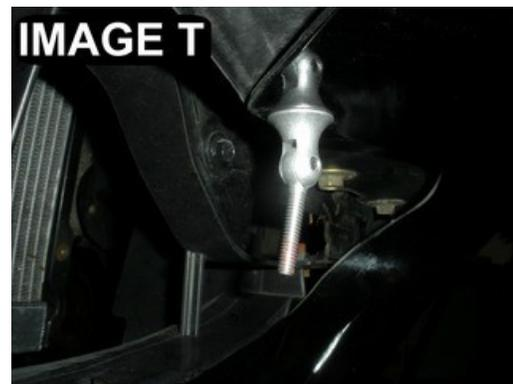
5. Once these upper mounts are secured, you can then mount the lower portion of the braces outward to the splitter. We left the mounting location your decision, but recommend the area where the front of the splitter curves out an extra inch. An easy trick is to paint the bolt head with a bright colored paint marker and while the paint is still wet, mark the spot where you want to drill. **(IMAGE U)**, **(IMAGE V)** and **(IMAGE W)**
