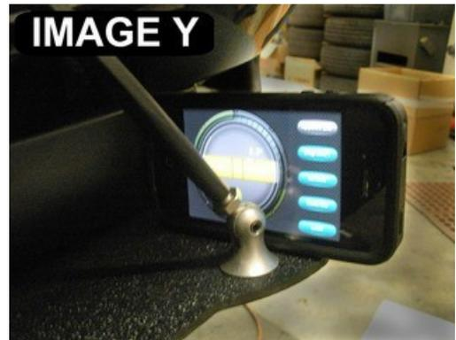
6. Again, make sure you're even on both locations, drill once! **(IMAGE X)** Install the supplied Allen head bolt to secure the brace to the splitter. Now you can extend the braces as you see fit. There is a lot of adjustment in them. You can use a level to fine tune the degree of angle to balance both sides. **(IMAGE Y)** Once you have them set, secure with the lock nut located on one side of the brace.
