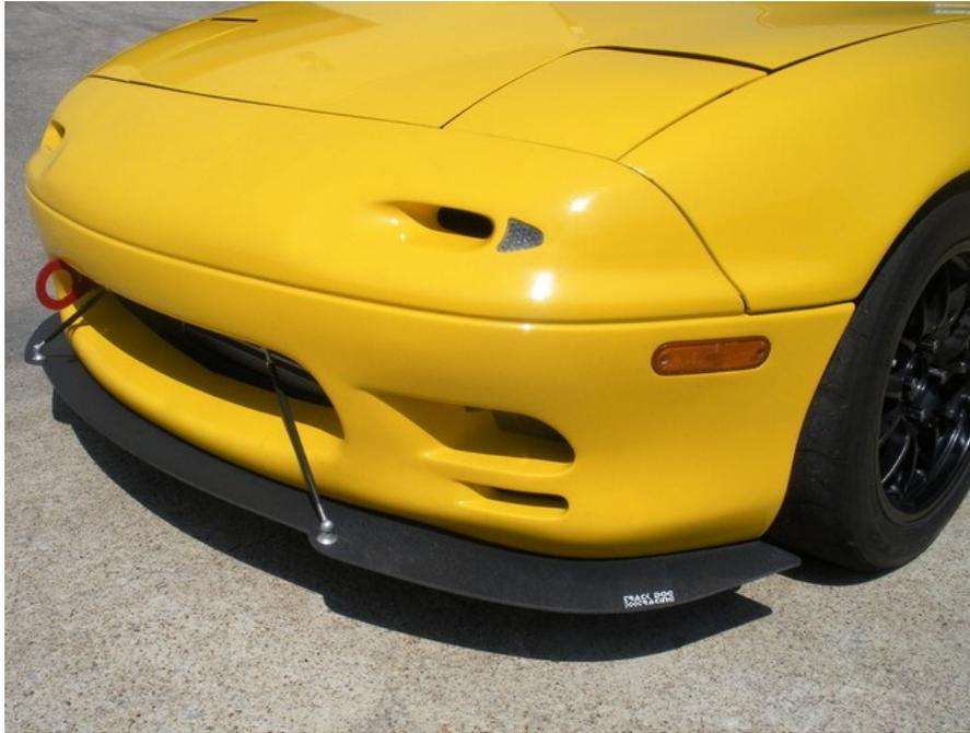
Thank you for purchasing the Track Dog Racing Radical Air Splitter/Protector. The Air Splitter is designed to help protect the Racing Beat Type II bumper by allowing the Air Splitter to slide over obstacles, such as steep driveways. The TDR Air Splitter is made from 3/16" thick, high-impact ABS plastic and will surprisingly take a lot of abuse. The textured top finish blends in well with any color.
